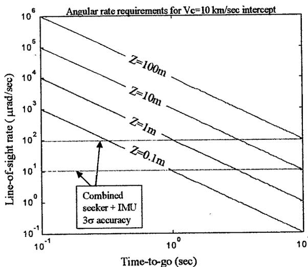
Figure 2 Line-of-sight rate for a 10 km/s closing target
