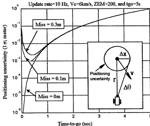
Figure 4b Required position measurement accuracy for generating independent LOS rate diagnostics
