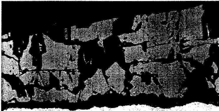
Figure 7 Micrograph Showing a Shallow, Oxide-filled Depression on the Internal Surface Magnification: 500x Etchant: Nital
