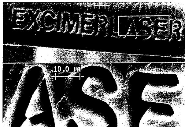
Figure 5. The words "EXCIMER LASER" ablated into a human hair.
