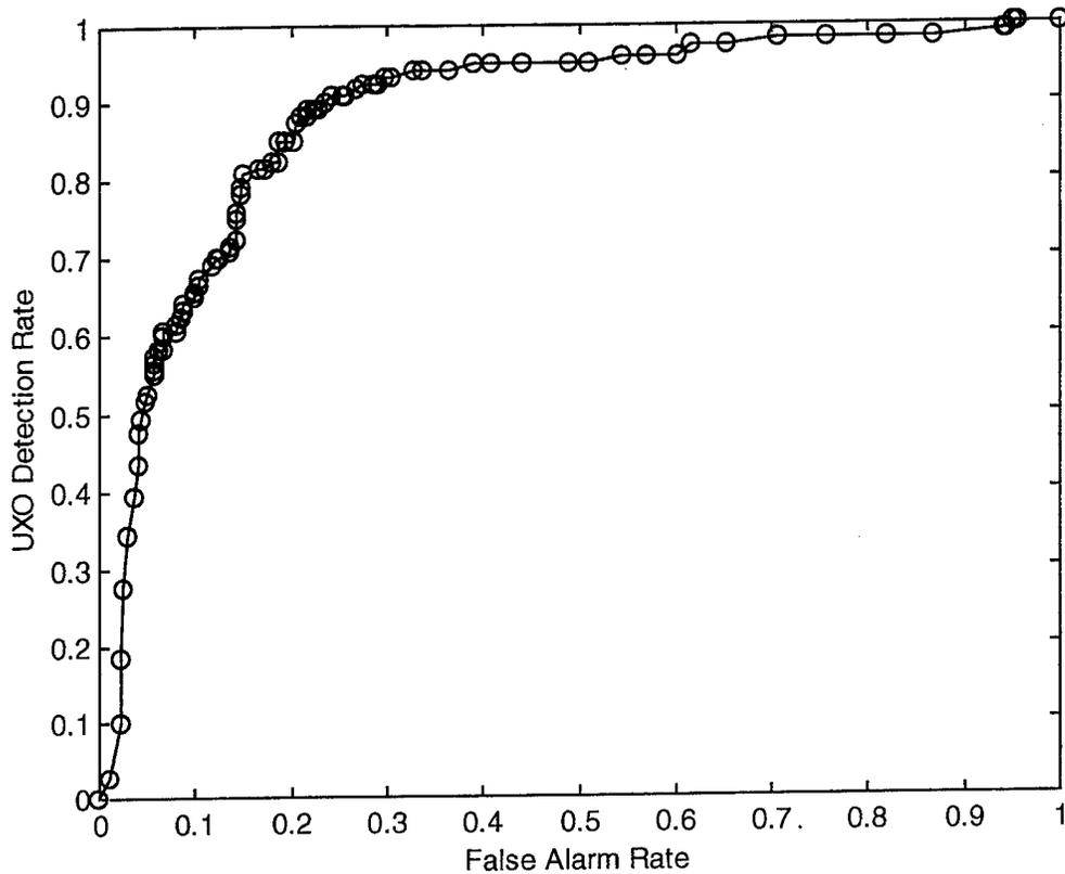
**Figure 20. Receiver operator characteristic curve for Buckley**
