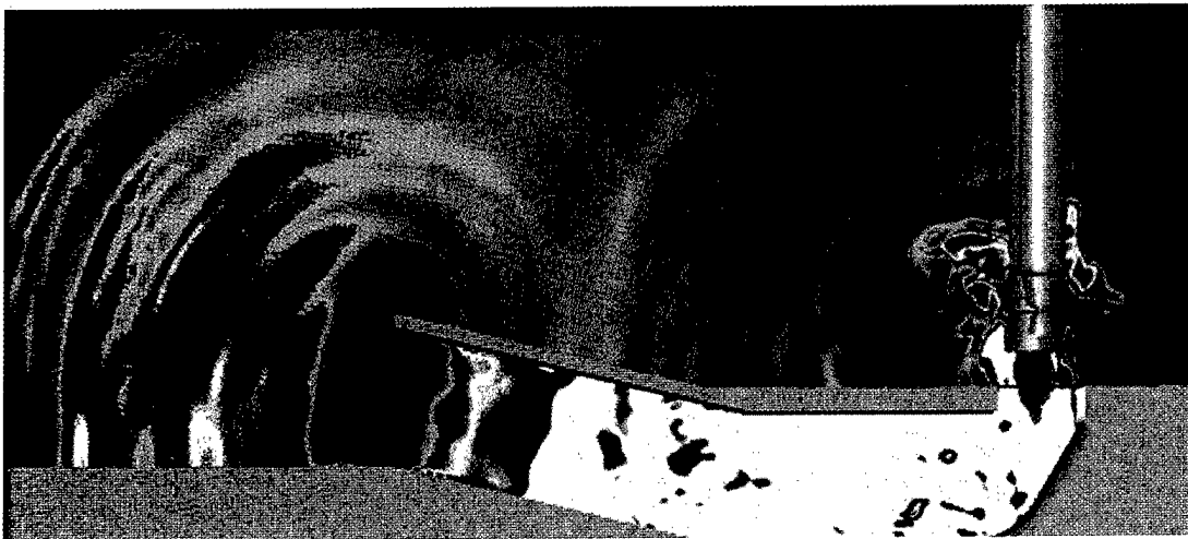
Snapshot of the pressure field around the launch duct at 290 ms after motor ignition. Both the initial waves, which progress axially up the vehicle, and the exit wave from the duct opening, which travels laterally back to the vehicle, are visible.
