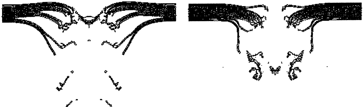
Damage in the [02/902] s laminate impacted by the flat rectangular rod ( h/w = 0.25 ) (left) and a thick rectangular rod ( h/w = 4.0 ) (right) at 4.0 km/s and 3.5 ms
