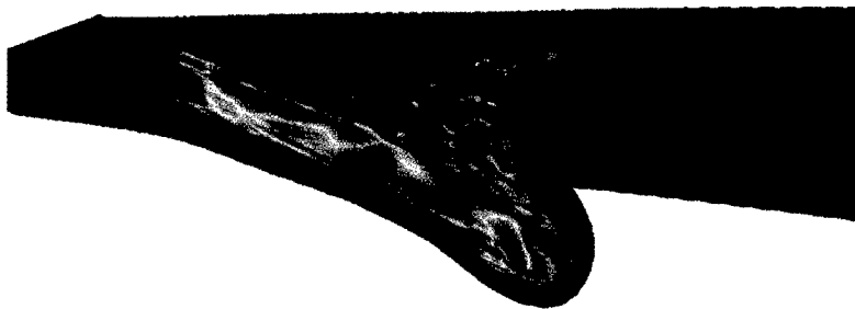
Long rod penetration with combined yaw and obliquity. Rod colored by pressure contours (blue, low pressure; red, high pressure).
