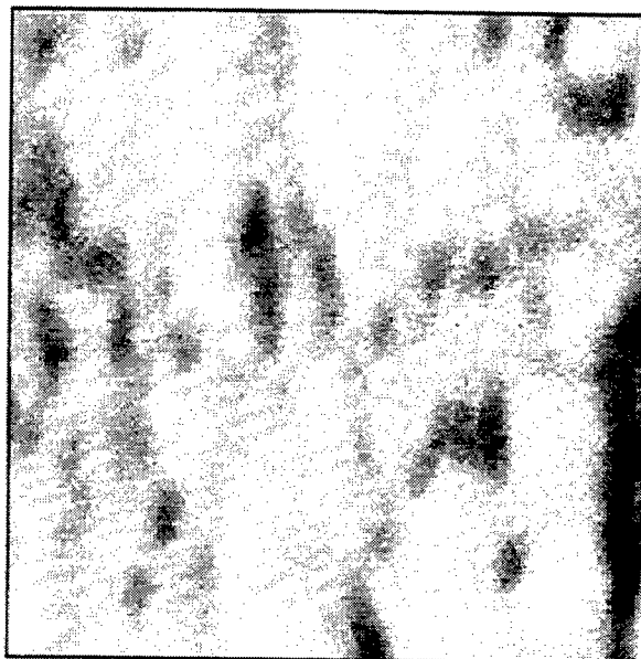
Figure 2b. SIMS image of \text{Li}^+ secondary ions on identical region in Figure 2a. The signal intensities are normalized to an 8 bit gray scale with black as the maximum signal. Acquired with a Cameca IMS 6f operating in the microprobe mode. Primary beam: \text{O}_2^+ , beam current 6 \times 10^{-12} \text{ A} , beam diameter: \approx 1 \mu\text{m} .
