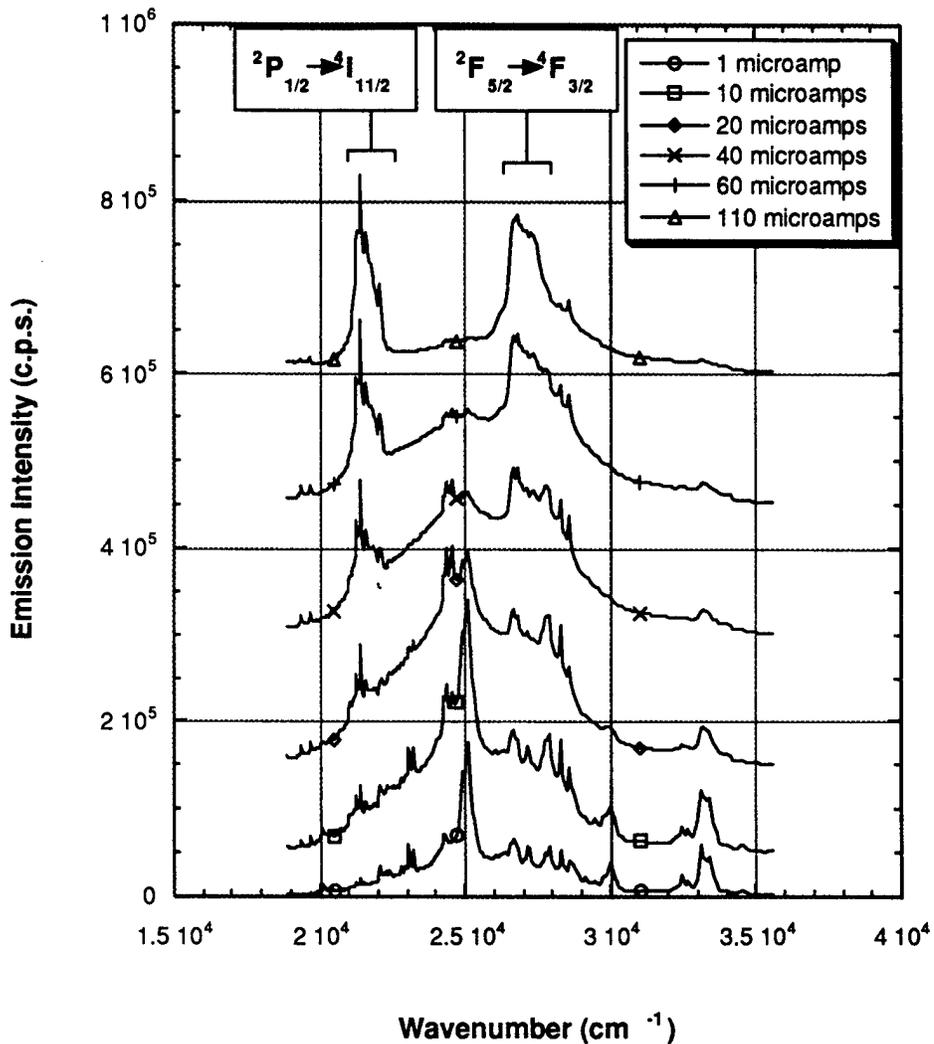
Figure 3. Nd emission excited by a 4 keV electron beam at various currents in Nd,Ce: $\delta$ -Al<sub>2</sub>O<sub>3</sub> nanopowders. Spectral redistribution and quenching behavior suggest the onset of stimulated emission above 20  $\mu$ A.
