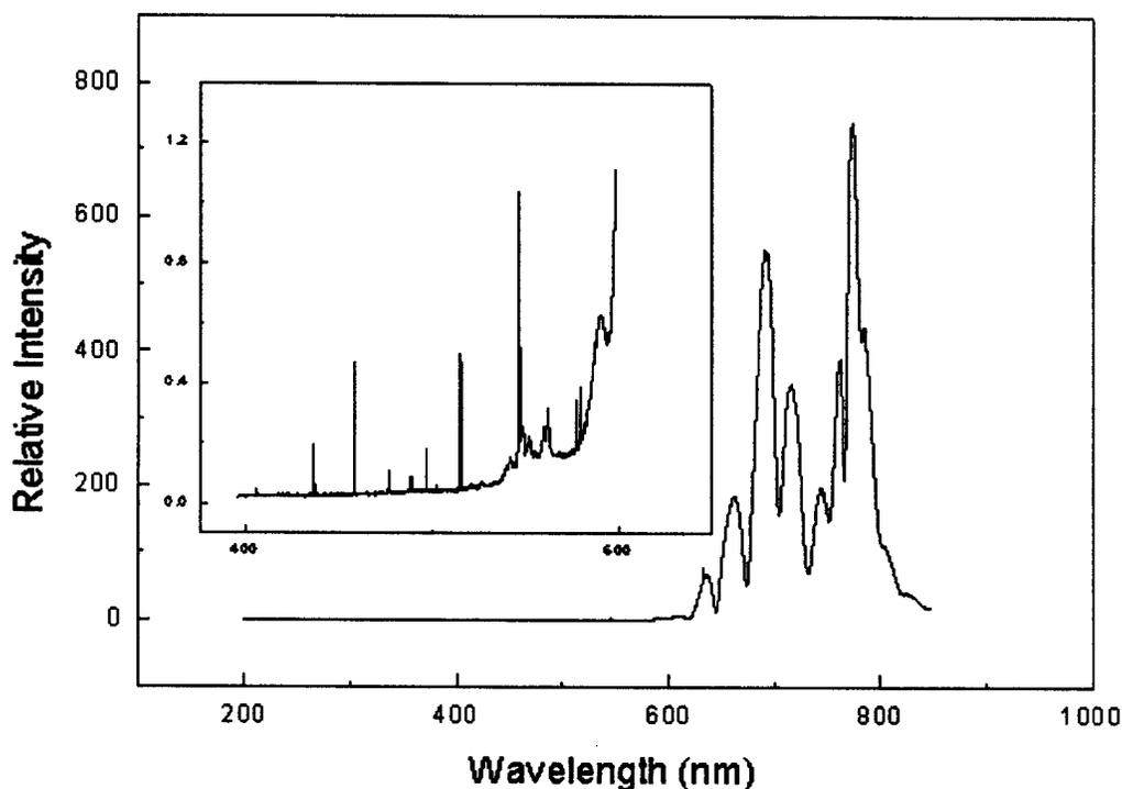
Fig. 2. Upconversion spectra of Nd,Ce:Al<sub>2</sub>O<sub>3</sub> nano-particles, with the laser tuned to a wavelength of 850 nm.
