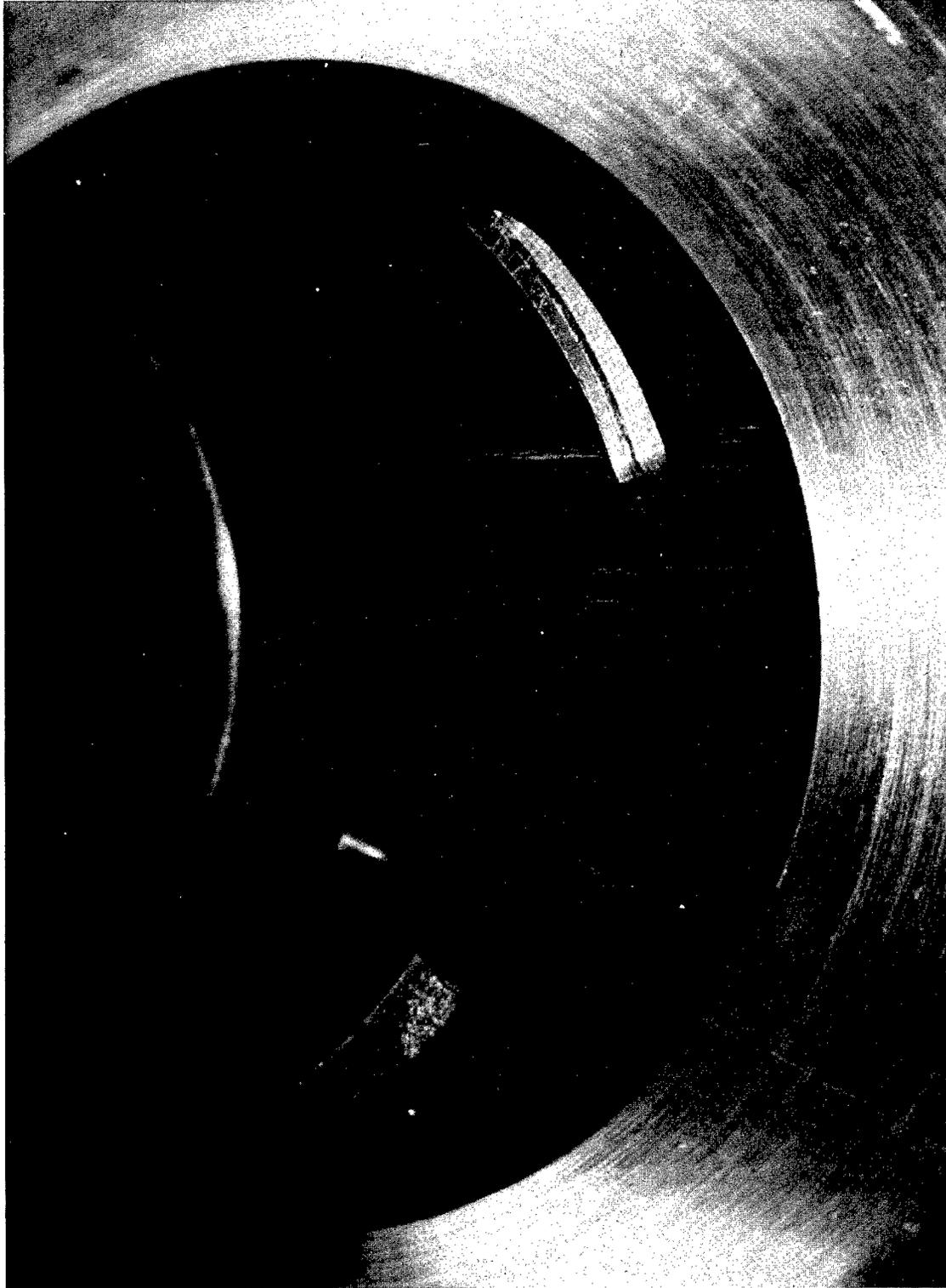
FIGURE 13. LIGHT SCORING ON INNER BEARING SURFACE OF M174 PISTON
