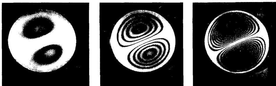
Fig. 6.12 Vibration contours on vibrating plate for various vibrating amplitudes (from Ref. 15).
