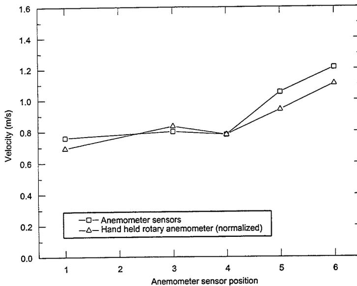
Figure 5. Comparison of hand held rotary anemometer with anemometer sensors for tree A3
