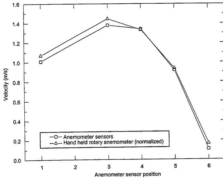
Figure 4. Comparison of hand held rotary anemometer with anemometer sensors for tree A2
