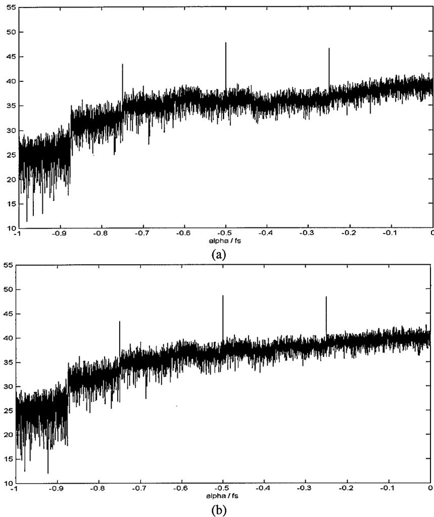
Figure 4-2.  $\lambda_E(\alpha)$  under  $H_1$  with  $SNR_{IN} = 0\text{dB}$  for: (a) Channel 1 and (b) Channel 2
