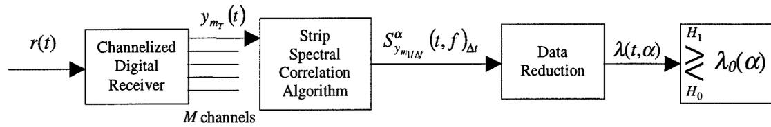
Figure 3-3. Channelized Cyclic Spectrum Analysis (CSA) Receiver
