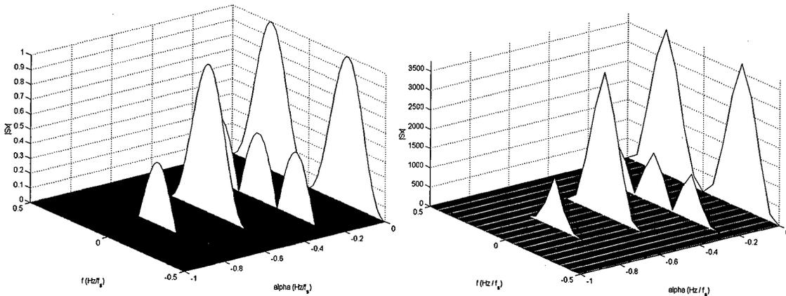
Figure 4-3. Summed Quadrature Receiver SCF: (a) Theoretical, and (b) Estimated
