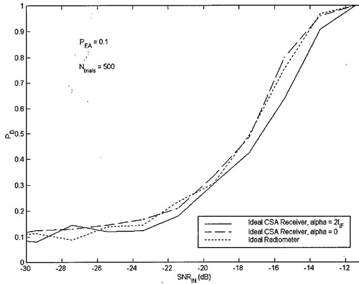
Figure 4-1. Ideal CSA Receiver Performance, Stationary Noise
