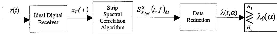
Figure 3-2. Ideal Cyclic Spectrum Analysis (CSA) Receiver
