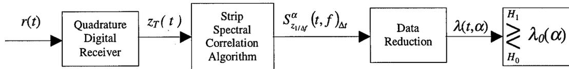
Figure 3-2. Quadrature Cyclic Spectrum Analysis (CSA) Receiver
