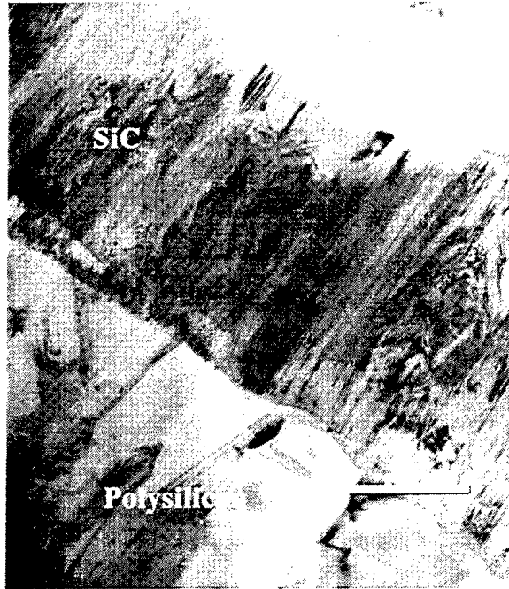
Figure 1- XTEM image of SiC (for high temperature applications) grown on as-deposited poly-Si (reference provided in text).
