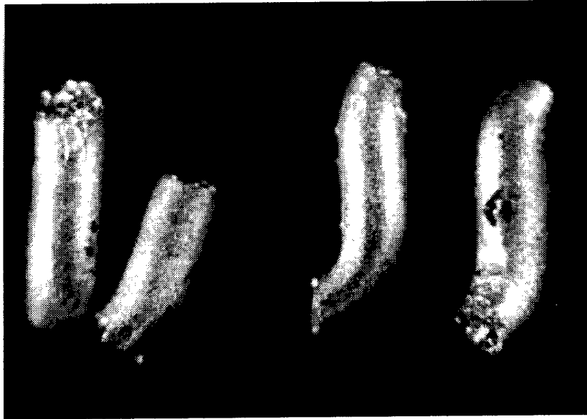
Figure 4. Photograph of four Pt-Ir wire fragments.
