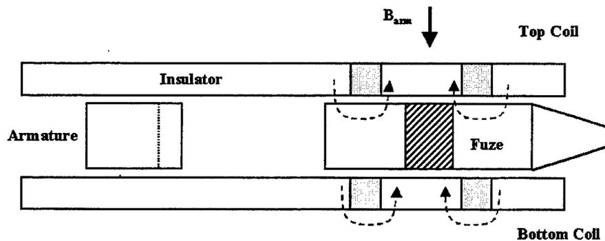
**Figure 15.** Schematic Illustration of the Active Shield Arrangement.
