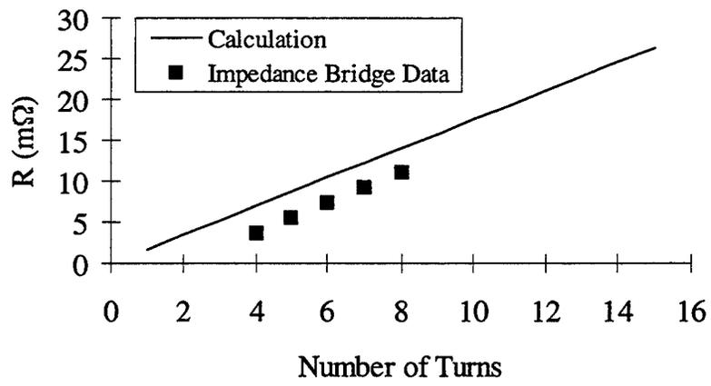
**Figure 18.** Inductance (Top) and Resistance (Bottom) for a Single Rectangular Coil as a Function of the Number of Turns.
