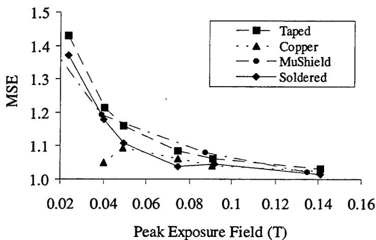
Figure 4. MSE Data for the 0.254 mm (0.01 in) Thick Materials.
