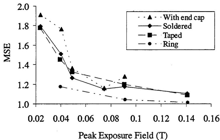
**Figure 3.** MSE Data for the 0.635 mm (0.025 in) Thick Materials.
