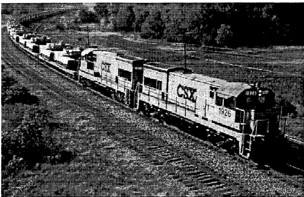
**Figure 6. Military Unit Train with M1A1 Abrams Tanks [Ref. 76]**
