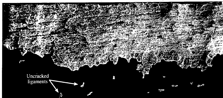
Figure 7. Interrupted tests demonstrate that high-temperature cracking occurs by fingers of decohesion that advance into uncracked material, with some uncracked ligaments remaining behind. As shown, the crack advanced from bottom to top with regions of intergranular cracking shown in black; all other areas are room-temperature transgranular fracture.
