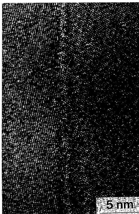
Fig. 2 HR-TEM image of a general GB in SiC which is viewed parallel to the beam. No amorphous film is found.
