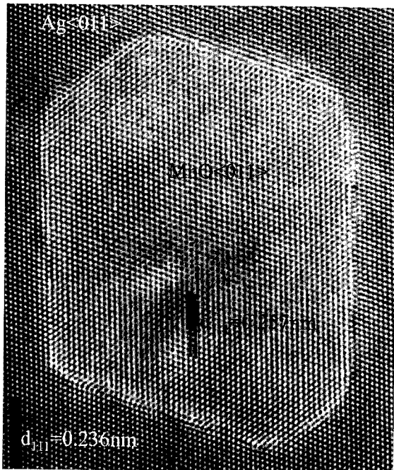
Fig.3 MnO precipitate in Ag as produced by internal oxidation followed by dissolution of 3 at.% Zn in the Ag matrix which reduces the Mn_3O_4 precipitates .
