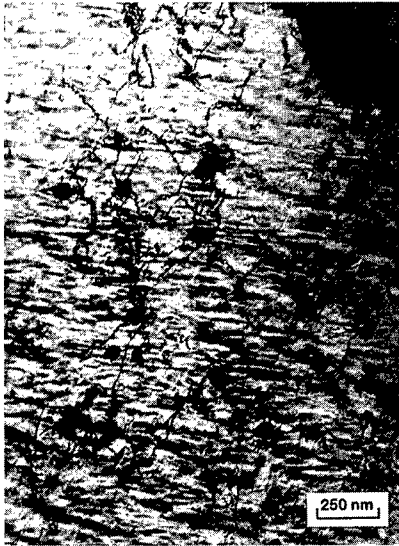
Fig.3. Structure of the Fe-32Ni alloy after the \alpha \rightarrow \gamma transformation during a slow heating at a rate of 0.2 deg./min. to 823 K (0.2 deg./min.)
