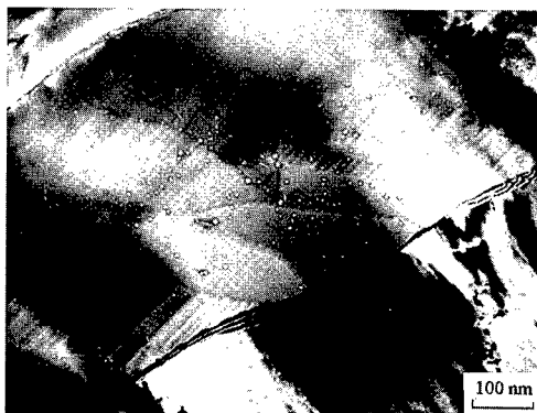
Fig. 3. Structure of the low-activation Cr13Mn7W2 steel after irradiation with 1.5-MeV \text{Kr}^+ ions up to the dose of 200 dpa at 650 °C.
