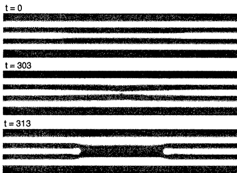
Fig. 2: Hole formation at the thinnest place in an individual layer (sample size 128 x 24; length and time units l_0 and t_0 ).
