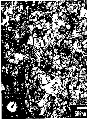
Figure 1. Typical microstructure of UFG Cu processed by ECA pressing.
