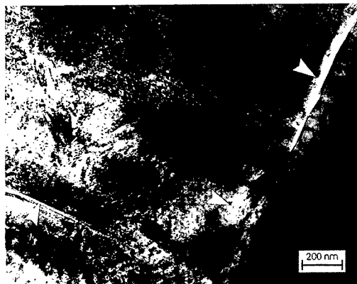
Figure 5. Cross sectional TEM micrograph of a TiN coating-substrate composite. The arrows show fractured zones due to rolling contact fatigue tests.
