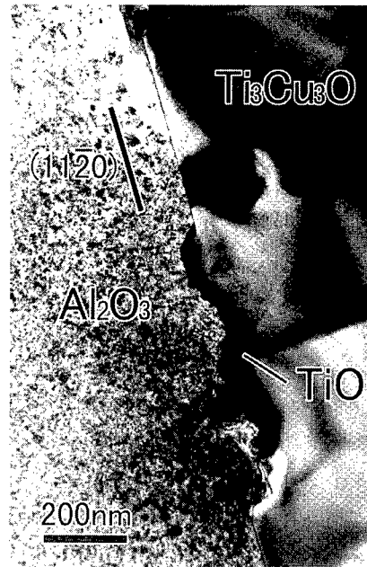
Fig.3 An atomically-flat Ti 3 Cu 3 O/sapphire interface where a continuous TiO layer is not present.
