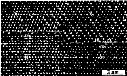
Fig. 7 [T10] HREM image of a four-layer step.
