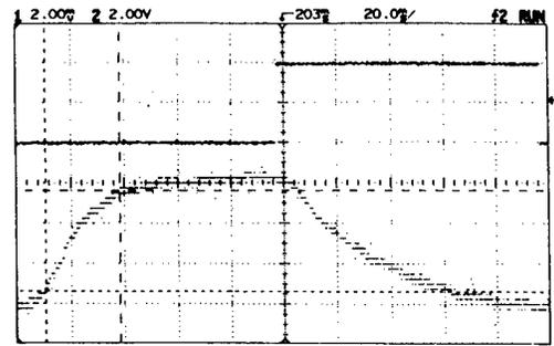
Fig. 3 Typical optical response curve for a 5 micron TN cell treated with an alignment layer
