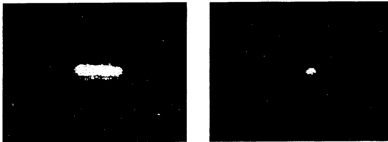
Fig. 5 : near field pattern 0.63\mu\text{m} of two channel waveguides at 0.63\mu\text{m} fabricated by wet etching. The cross sections are 50\times 2\mu\text{m}^2 (left picture) and 10\times 2\mu\text{m}^2 (right)
