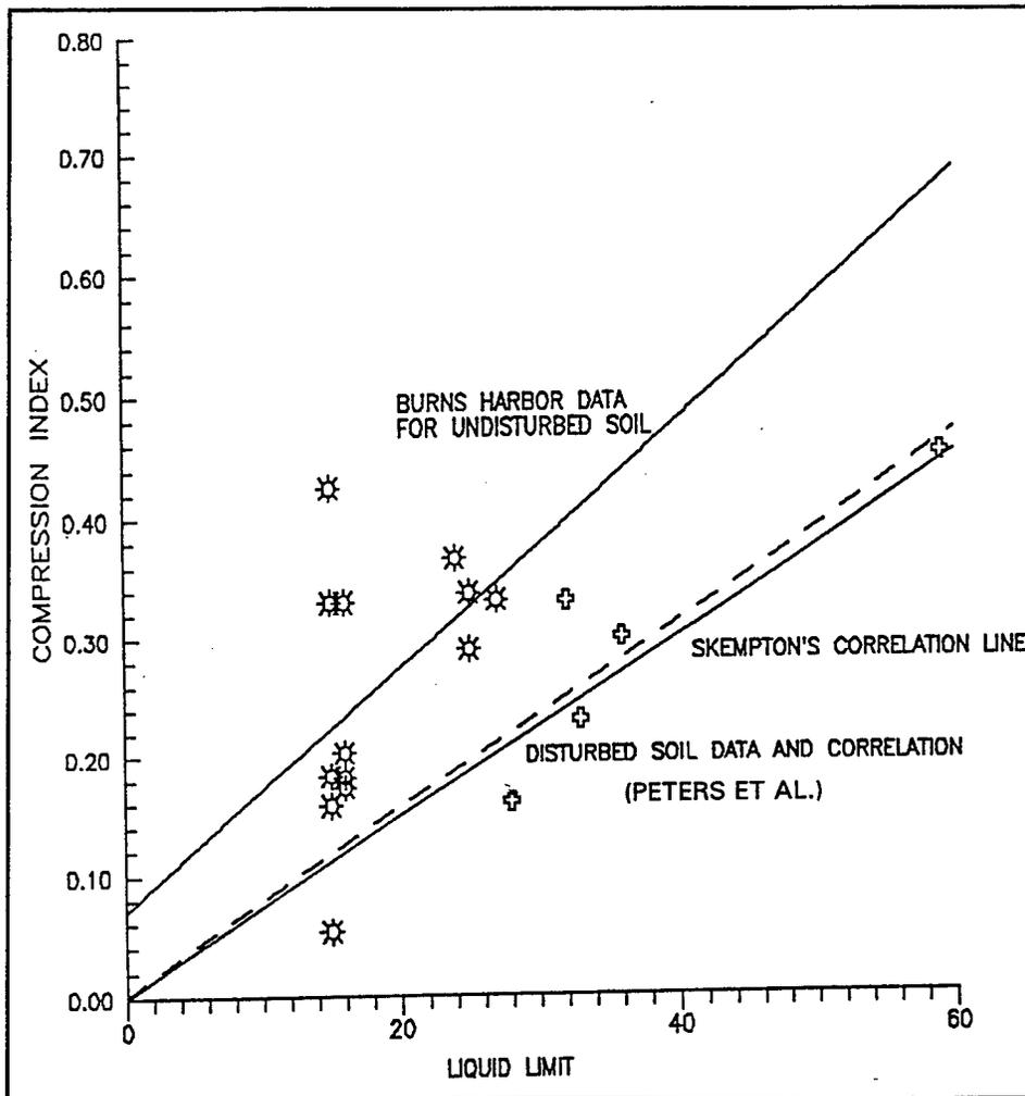
Figure 4-18. Comparison of Skempton (1944) and project soil data
