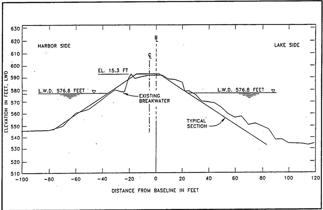
Figure 4-21f. 1985 Survey cross section, Station 34 + 00
