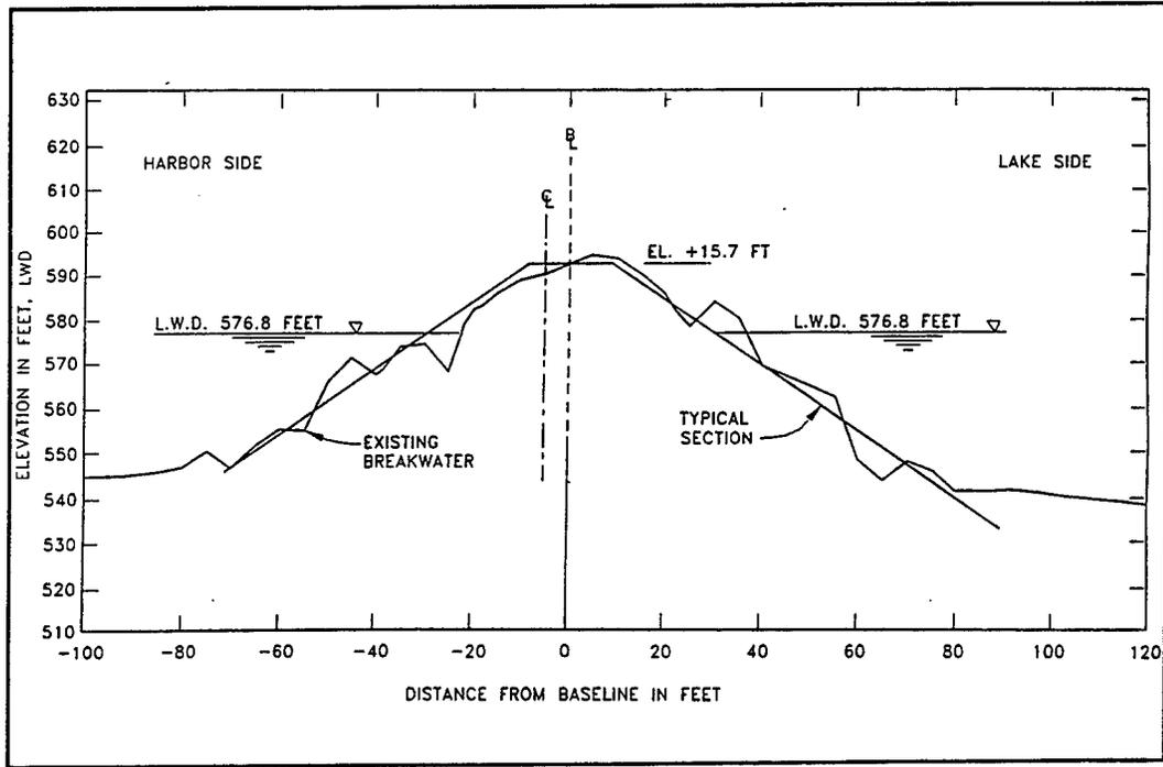
Figure 4-21a. 1985 Survey cross section, Station 23 + 00
