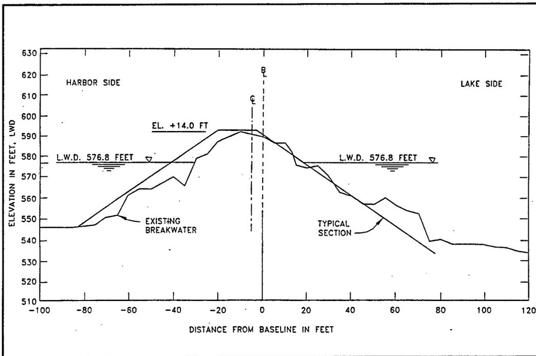
Figure 4-21d. 1985 Survey cross section, Station 29 + 00
