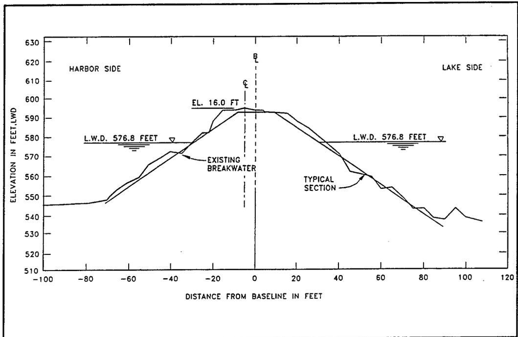
Figure 4-21b. 1985 Survey cross section, Station 24 + 00
