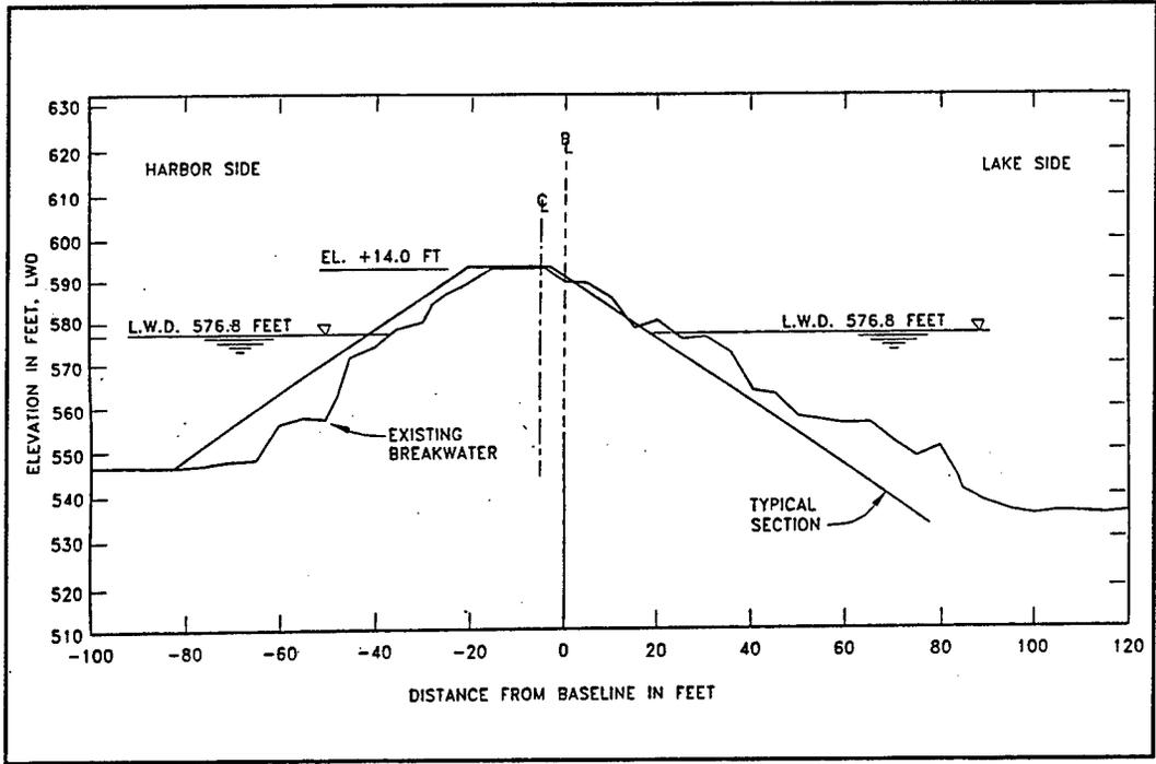
Figure 4-21e. 1985 Survey cross section, Station 32 + 00
