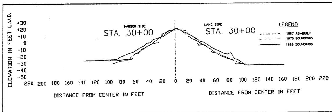
Figure 5-4. 1989 breakwater profile showing distortion below waterline
