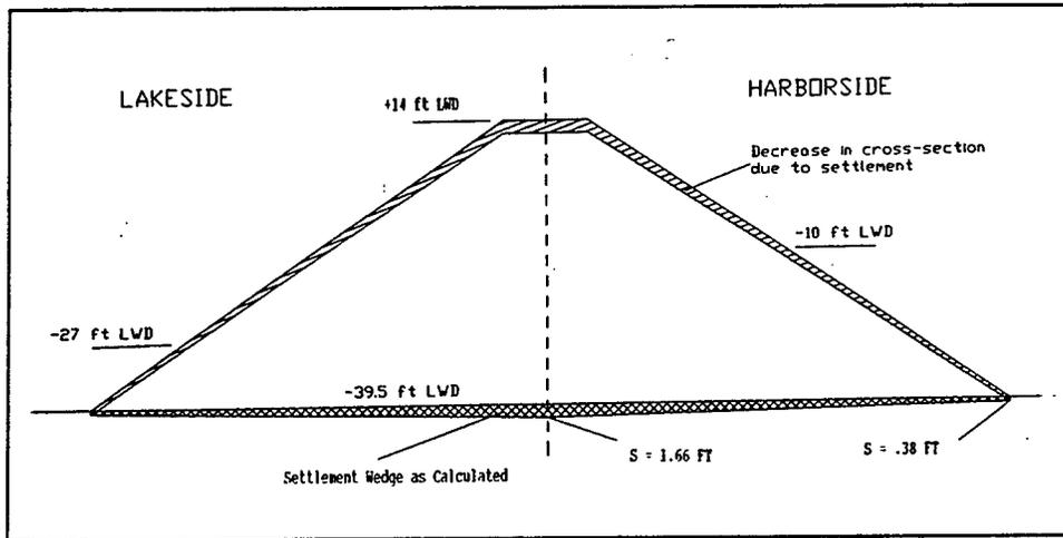
Figure 5-11. Expected cross-section adjustment due to settlement
