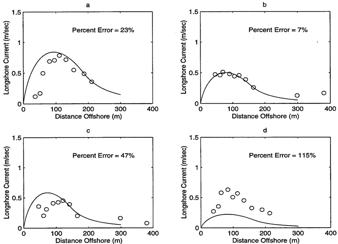
Figure 9. Plot of the predicted (line) and measured (circles) longshore current for DUCK94
