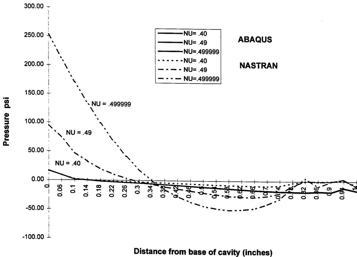
Figure 3. Plot illustrating the hydrostatic pressure stresses in the VEM from linear elastic analyses .
