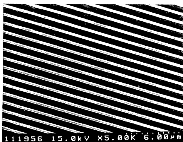
Fig.1, SEM image of the \text{Al}_2\text{O}_3 grating prepared by sol-gel process.
