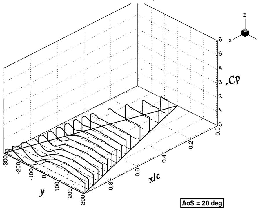
Figure 34: Surface pressure for  $\beta = 20 \text{ deg}$
