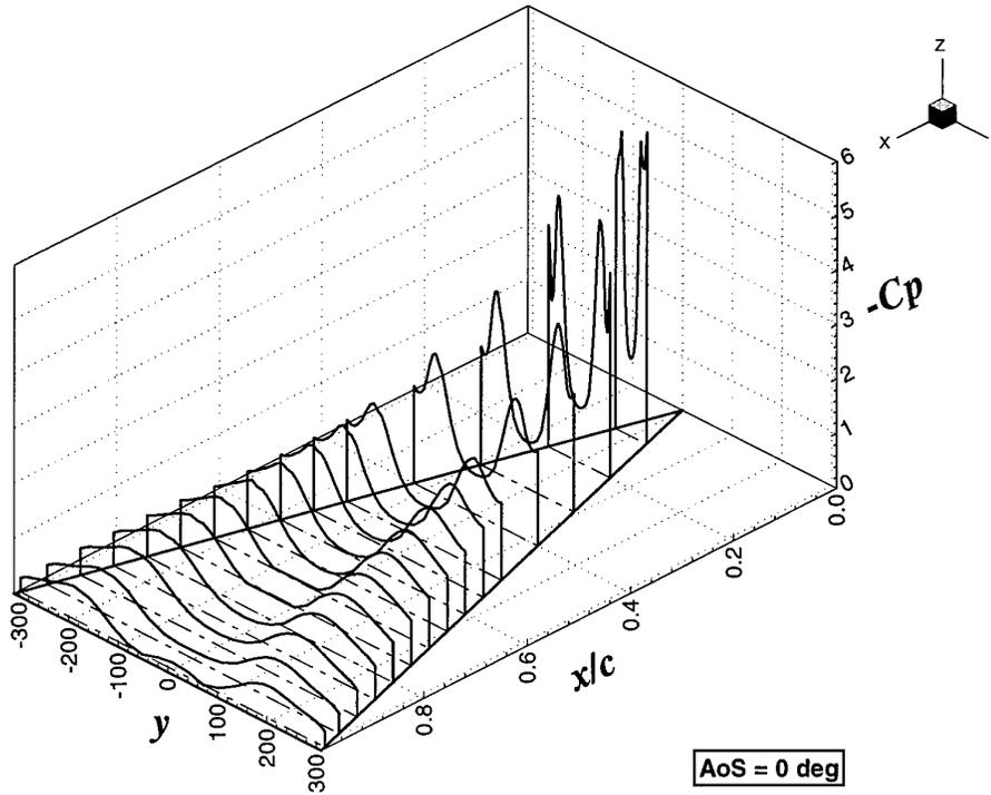
Figure 29: Surface pressure for  $\beta = 0 \text{ deg}$
