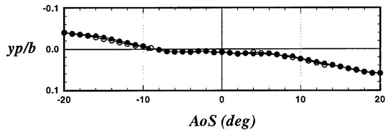
b. Effect of  $\beta$  on lateral position of center of pressure
