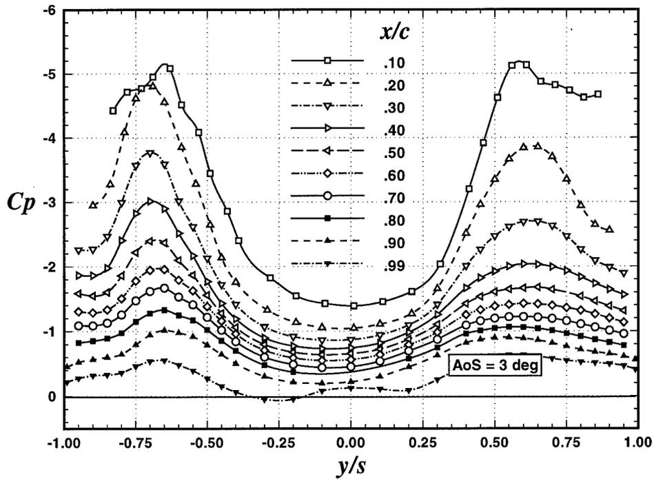
Figure 30: Surface pressure for  $\beta = 2$  and 3 deg
