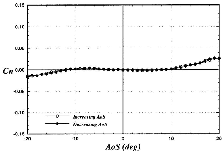
Figure 39: Effect of  $\beta$  on yawing-moment coefficient (data set 1)
