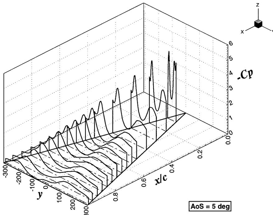
Figure 31: Surface pressure for  $\beta = 5 \text{ deg}$
