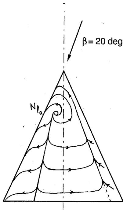
Figure 27: Conjectured topology of flow for  $\beta = 20$  deg
