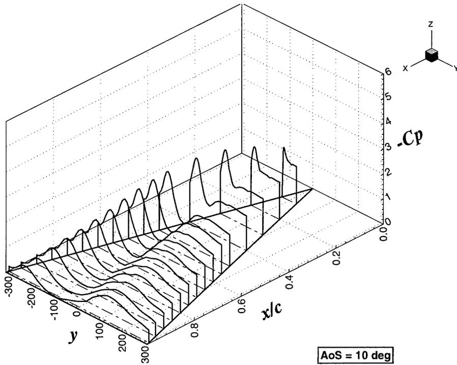
Figure 32: Surface pressure for  $\beta = 10 \text{ deg}$
