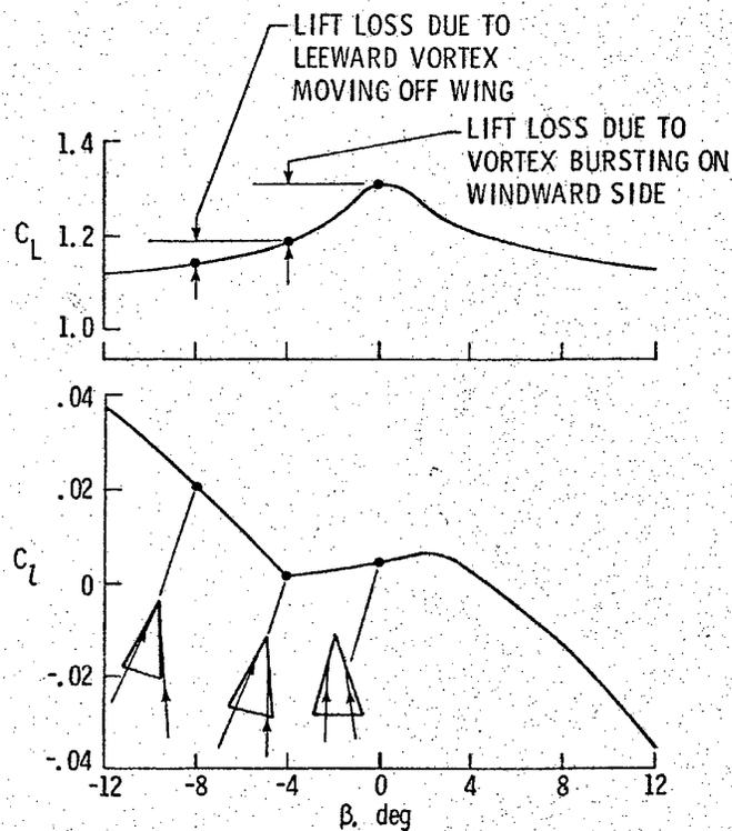
Figure 5: Effect of  $\beta$  on lift and rolling-moment coefficient of a 70-deg delta wing at  $\alpha = 36$  deg (Johnson, et al [5])
