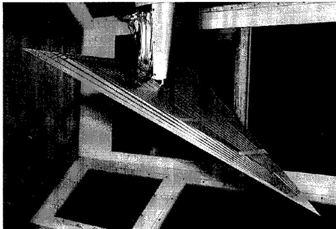
Figure 17: Delta wing with pressure taps in LTT
