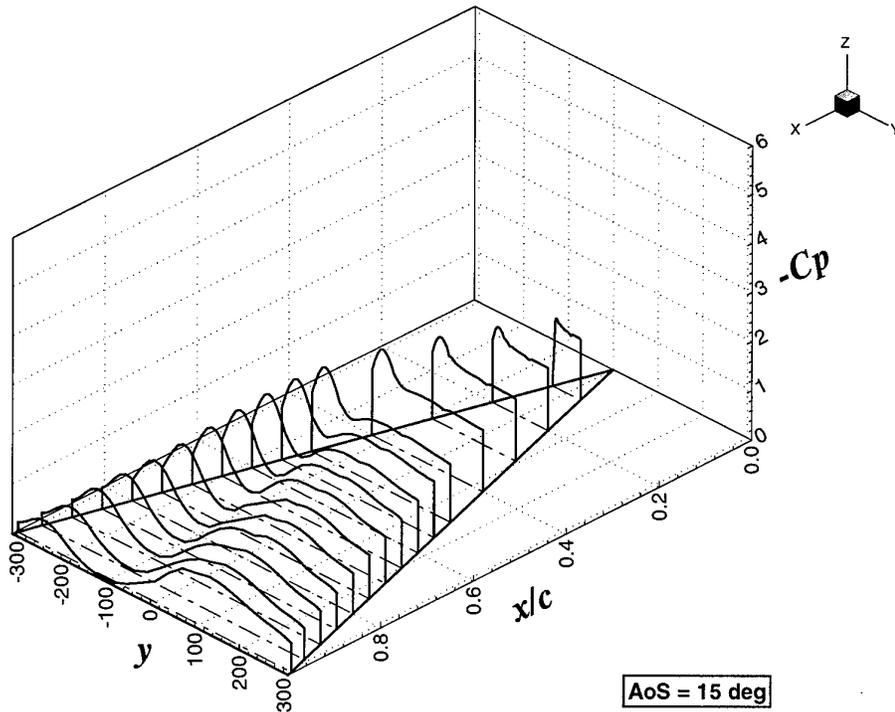
Figure 33: Surface pressure for  $\beta = 15 \text{ deg}$
