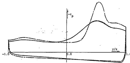
Figure 12: Effect of burst on spanwise pressure distribution near trailing edge of a 76-deg delta wing at  $\alpha = 21$  deg (Verhaagen and Naarding [7]); the dashed line represents the  $C_p$ -curve upstream, the solid line downstream of the burst location.
