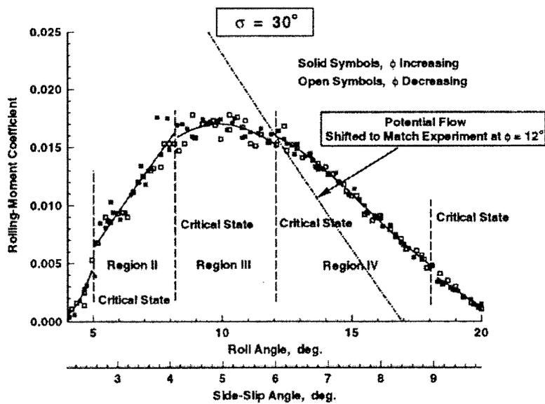
Figure 2: Effect of  $\phi$  on rolling-moment coefficient
