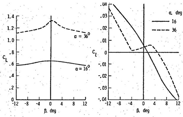
Figure 3: Effect of  $\beta$  on lift and rolling-moment coefficient of a 70-deg delta wing at low and high  $\alpha$  (Johnson, et al [5])
