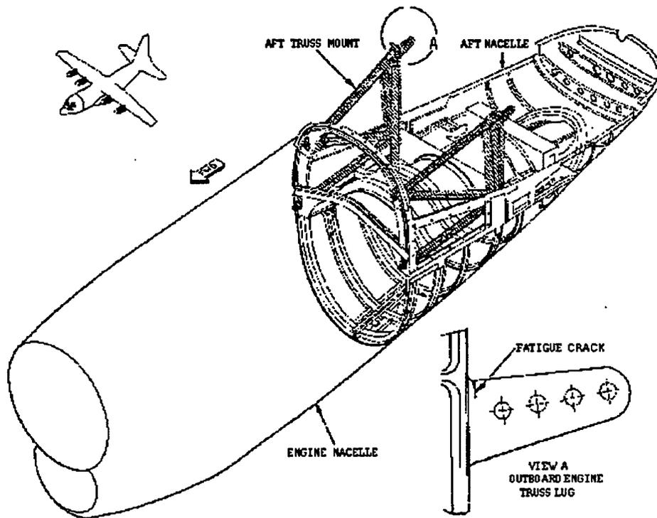
Figure 2-1 - Engine Aft Truss Mount Upper Tang Crack Location
