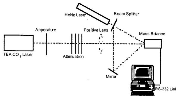
Figure 20. Experimental setup for measuring tissue mass-loss.
