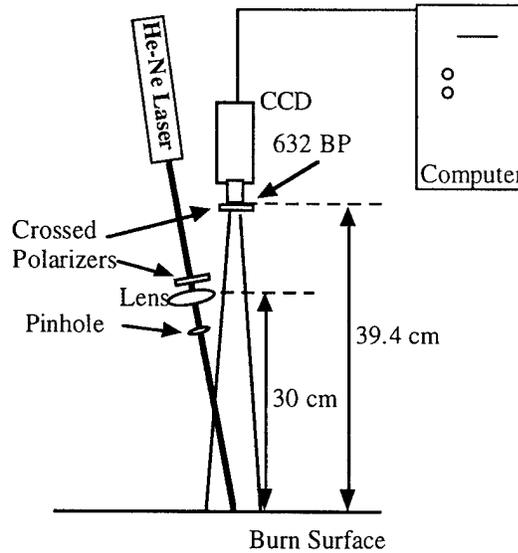
Figure 11. Experimental setup used to acquire speckle images. A HeNe laser is used as the source. The laser beam is focused onto to the object by the 30 cm focal length lens. The bandpass filter is used to reduce the effect of room light.
