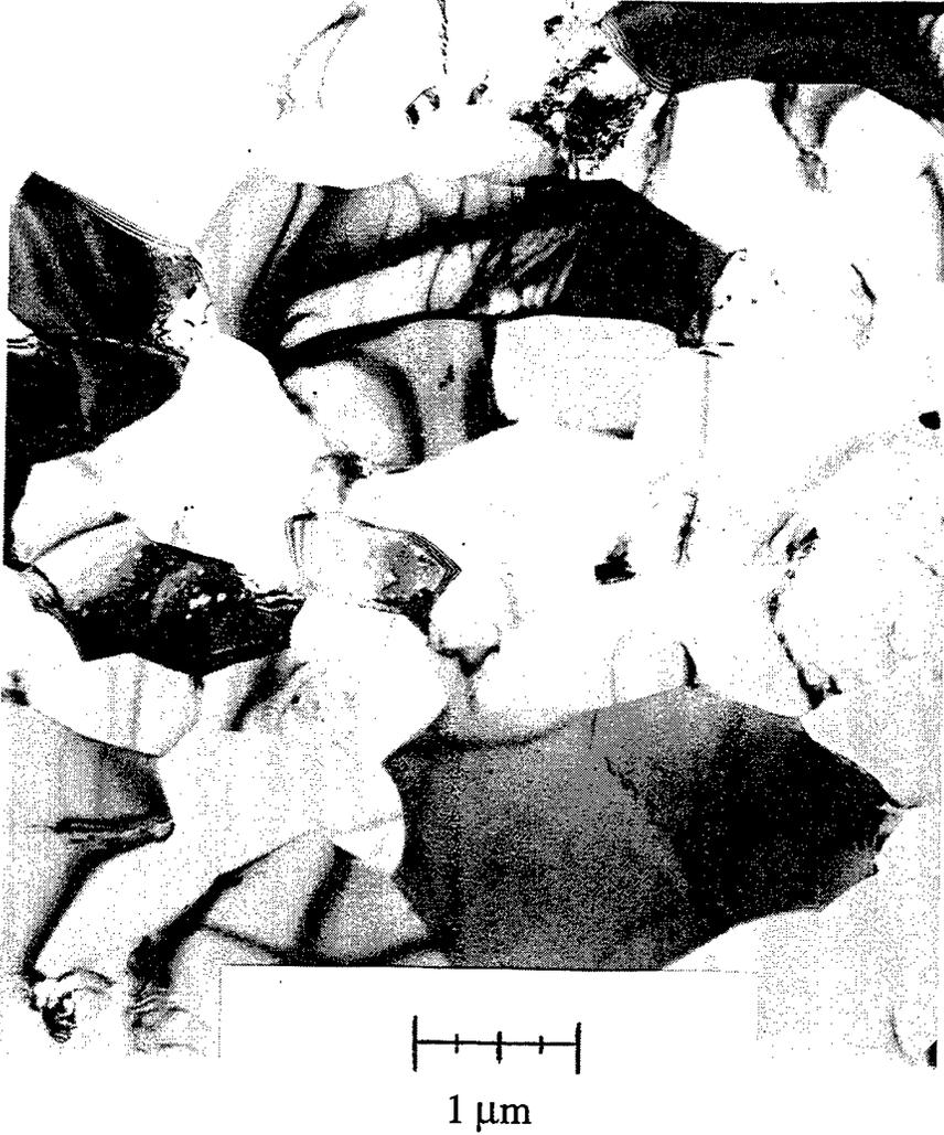
Figure 5.3. TEM micrograph of the sample processed by route A through 12 pressing operations (y plane)
