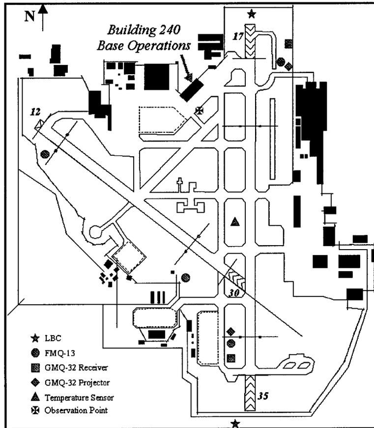
**Figure 2.1:** Location of weather sensors on Tinker Air Force Base. The location of the Base Weather Station (BWS), situated in Building 240, is also indicated as well as the “official” observing point, ☒.
