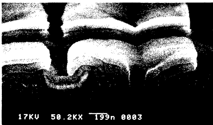
Photograph 6 SEM view of 0.3- \mu m-rule cell
