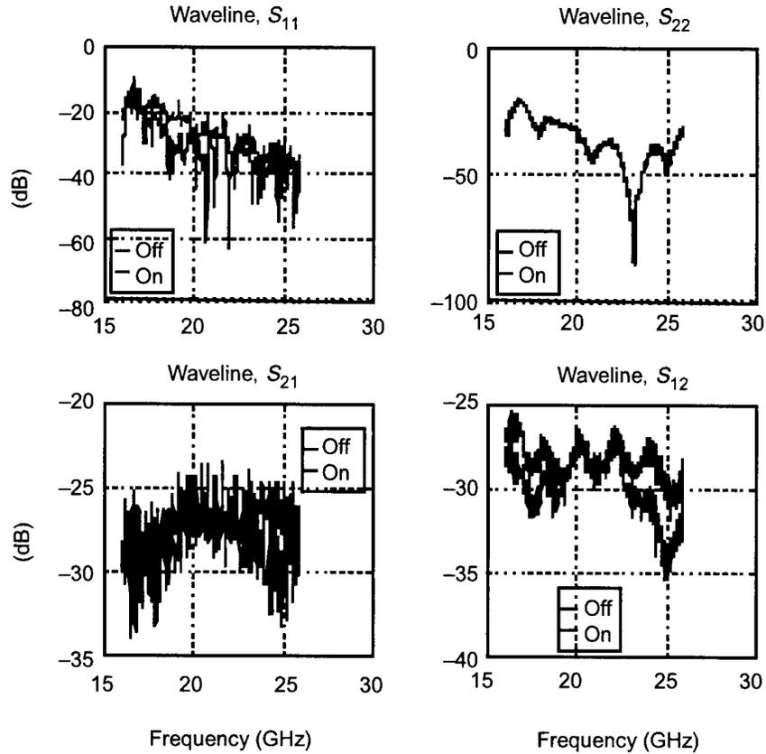
**Figure A-6. Waveline 18–26 GHz derivative of the two-port phase measurement.**
