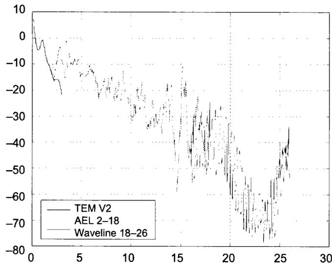
**Figure 9. Effective length of TEM V2 antenna.**
