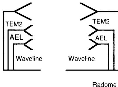
points for all three antennas. In this configuration, we measured the magnitude and phase of the TEM V2 antennas for the frequency range 0.045 to 10 GHz. This procedure was then repeated at the appropriate bands for the AEL and Waveline antennas.
