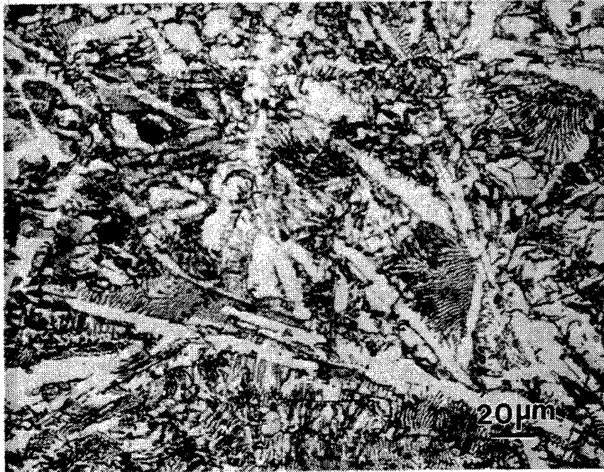
Figure 5.4. Microstructure of spray-formed Ta-Fe alloy. (a) Upper section, (b) lower section of the deposit.
