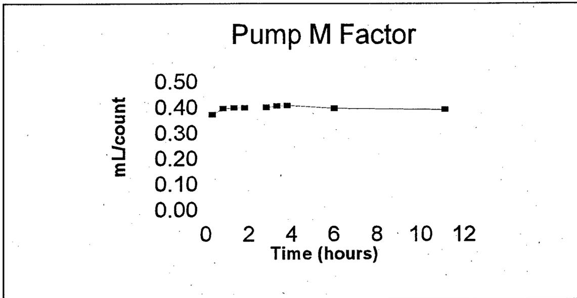
Figure 3.4. Pump factor constancy over 11-hour period
