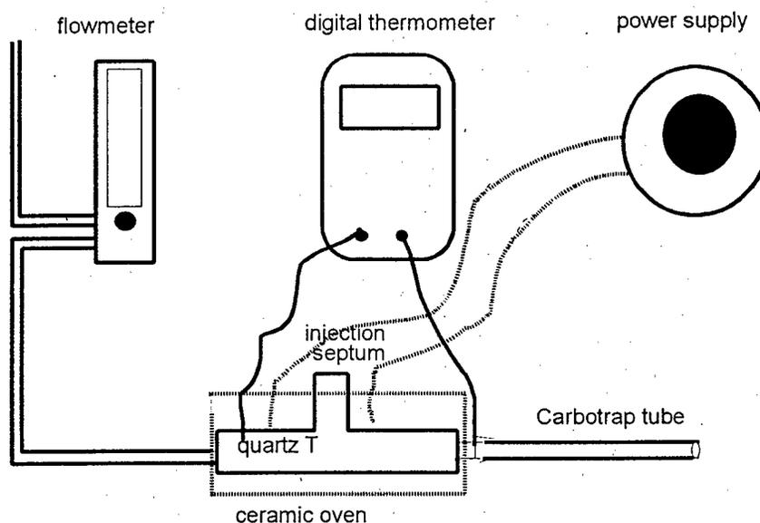
**Figure 3.1.** Calibration device for the TD/GC/MS sampling tubes. Samples are "pushed" onto the trap by a helium carrier gas flow from the flowmeter, but beyond that, sorbed in an analogous manner to field samples.
