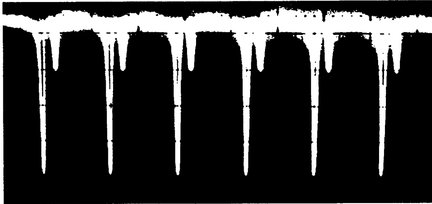
Figure 3: Oscilloscope trace of the synchronized output at the fundamental frequency of 3.3898 MHz. The smaller pulses are the input signal from the actively modelocked ring laser, while the larger pulses are the MQW laser's synchronized output.
