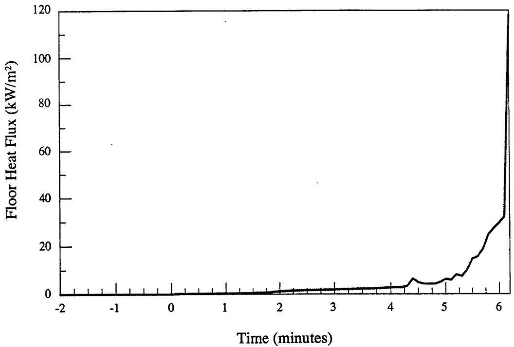
Figure A.3.c - Material # 3 - Floor heat flux vs. time
