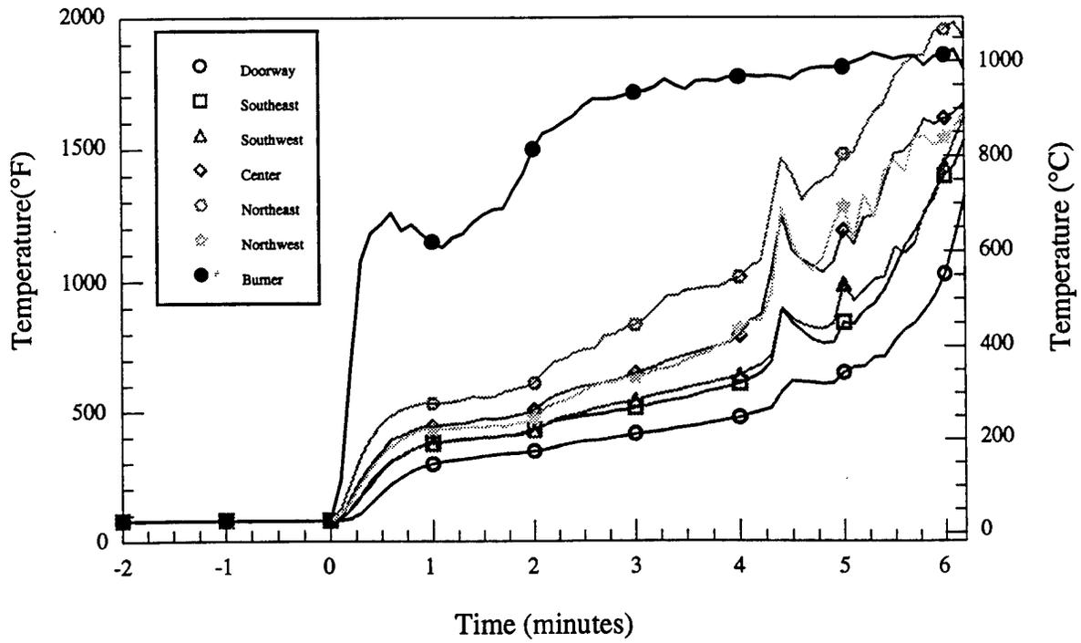
Figure A.3.d - Material # 3 - Room temperatures vs. time
