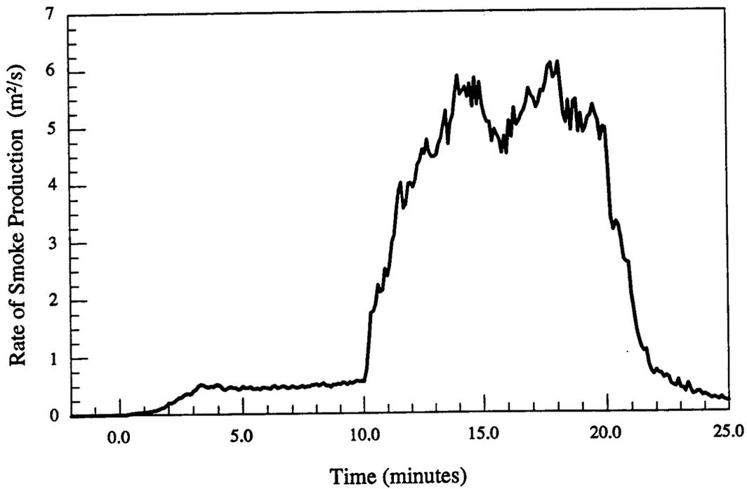
Figure 6.b - Material # 6 - Smoke production rate vs. time
