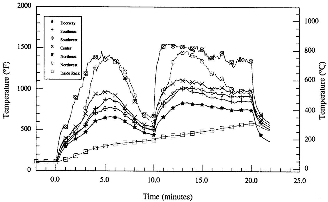
Figure 11.d - Material # 3 - Luggage rack - Room temperatures vs. time
