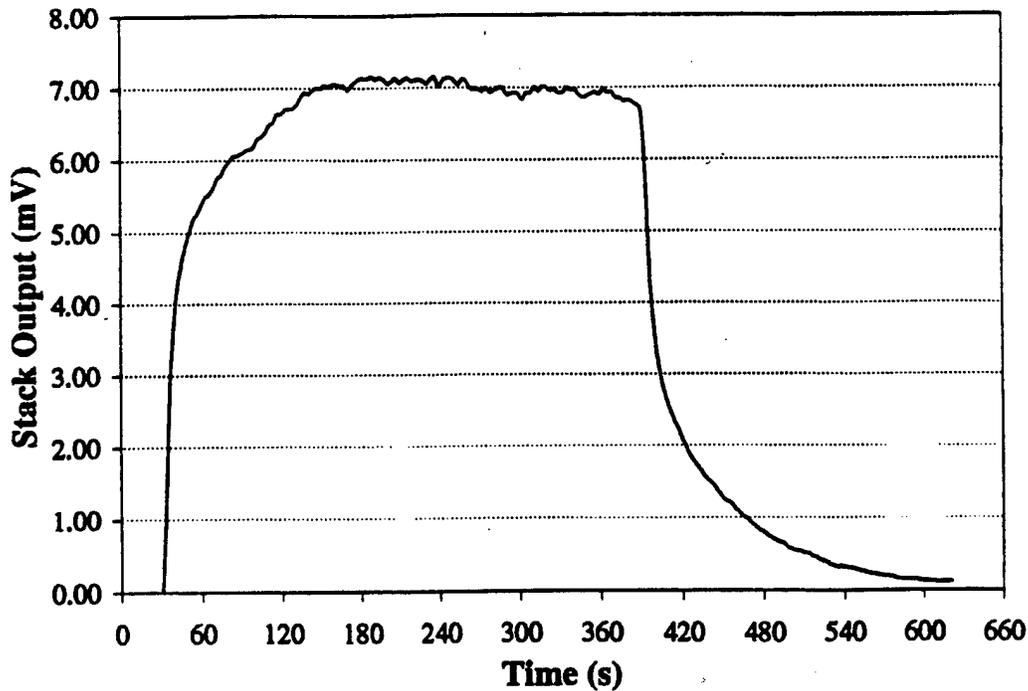
**Figure 6.3 – Stack Response to a 7 kW Thermal Pulse**
