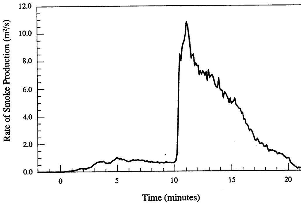
Figure 1.b - Material # 1 - Smoke production rate vs. time
