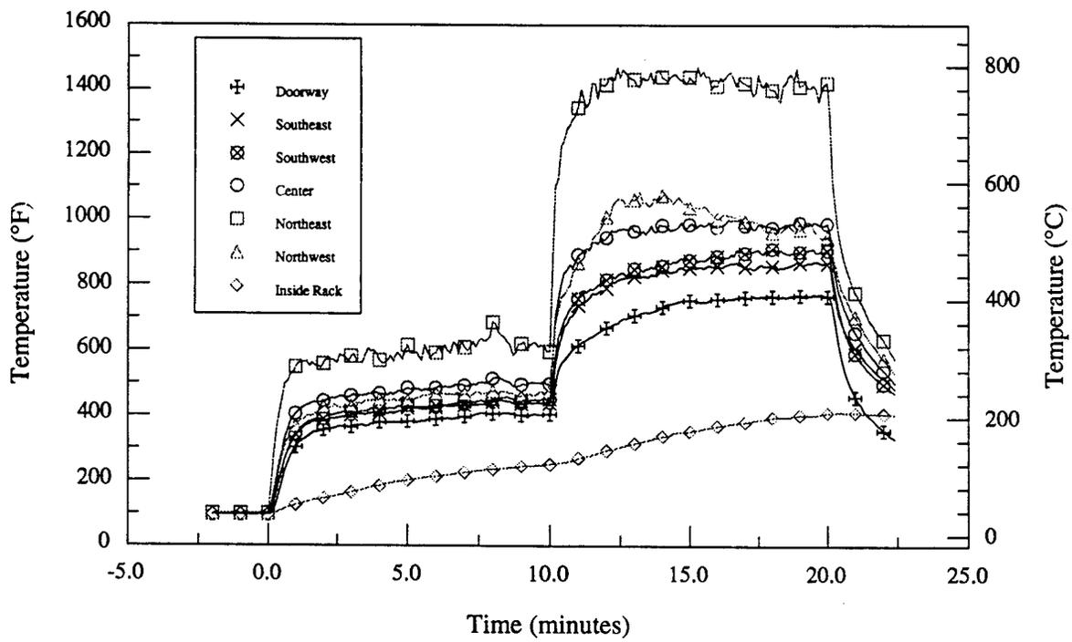
Figure 12.d - Material # 4 - Luggage rack - Room temperatures vs. time
