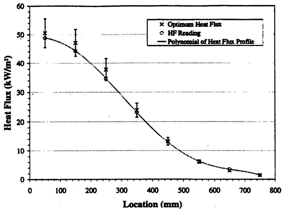
Figure 6.2 – Heat Flux Profile as a Result of Thermal Adjustment of Panel Operating Levels
