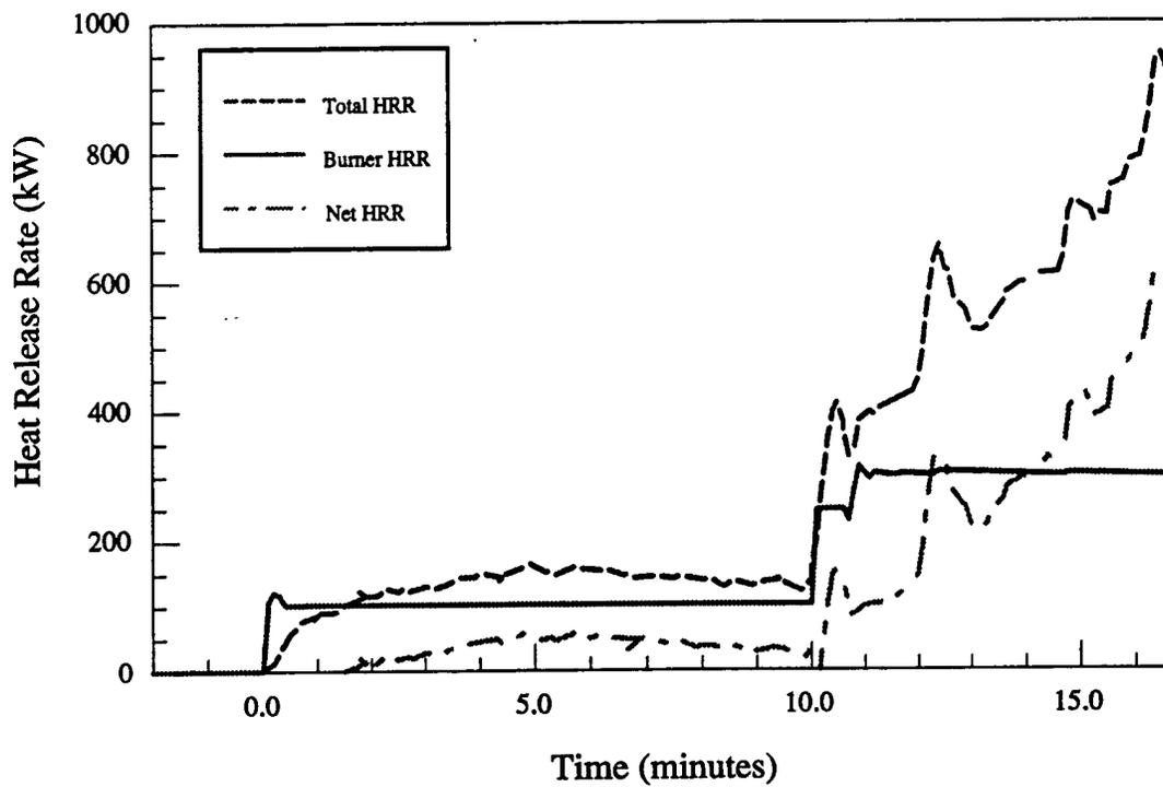
Figure 5.a - Material # 5 - Heat release rate vs. time
