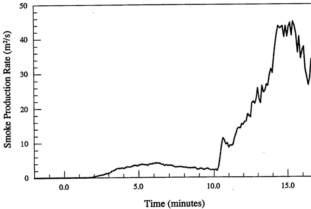
Figure 5.b - Material # 5 - Smoke production rate vs. time
