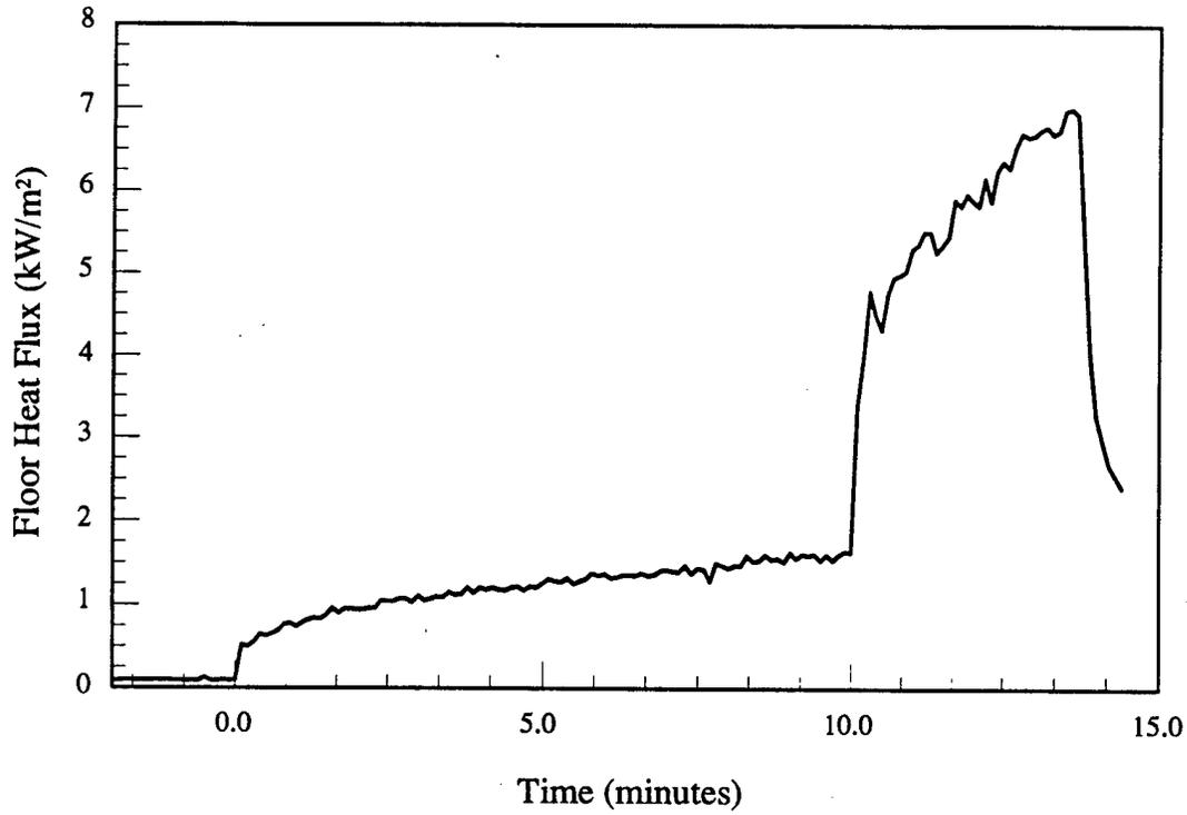
Figure 10.c - Material # 1 - Luggage rack - Floor heat flux vs. time
