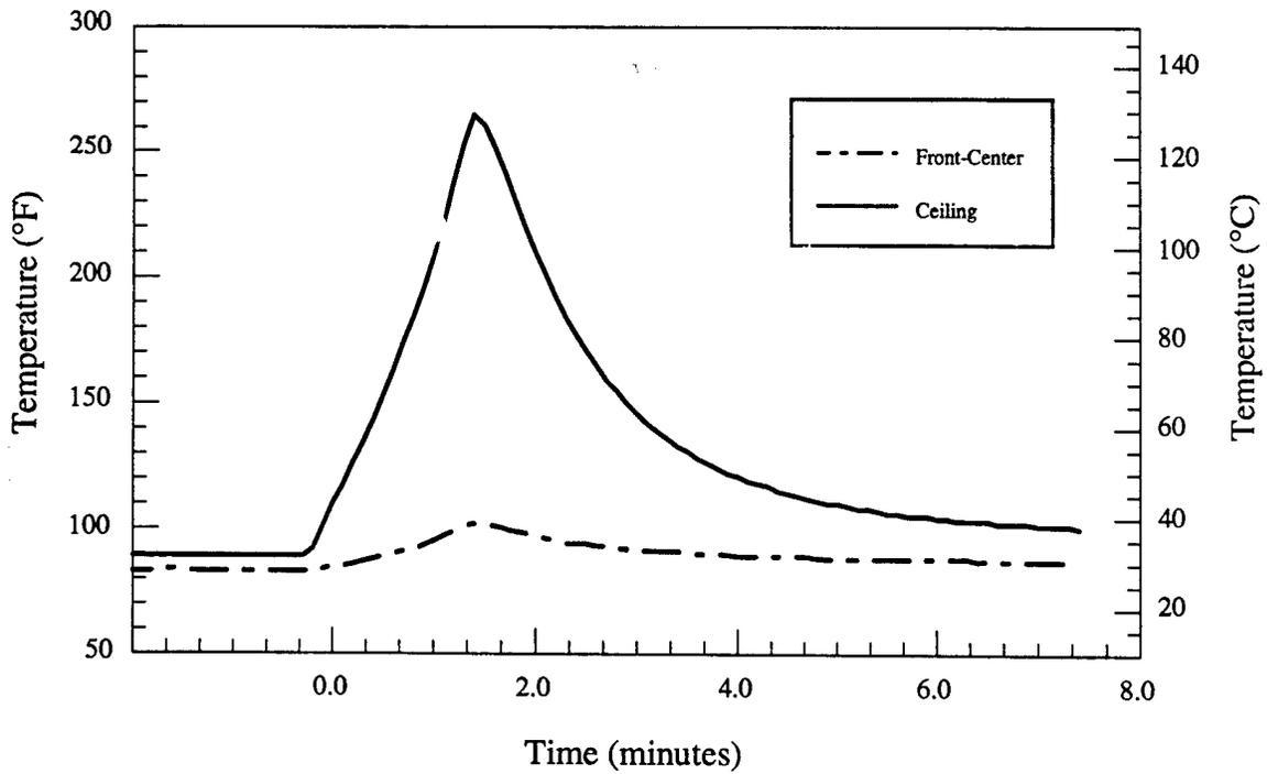
Figure 6.d - Material # 4 - Single chair - Room temperatures vs. time
