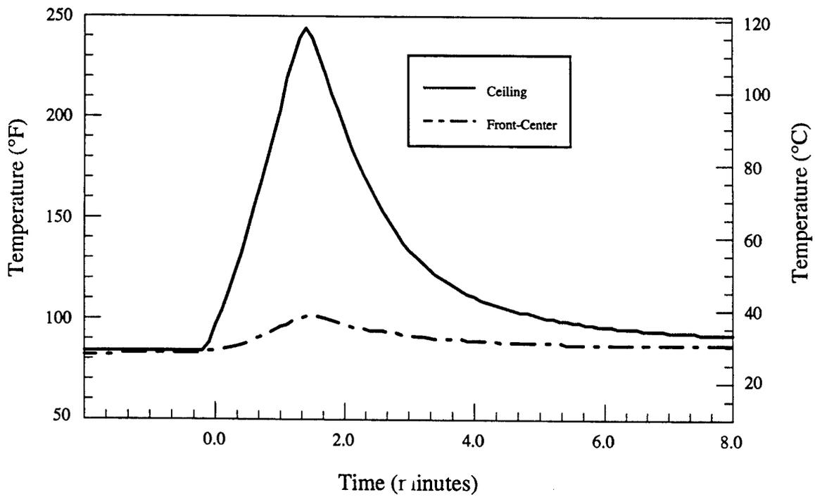
Figure 1.d - Steel - Single Chair - Room temperatures vs. time
