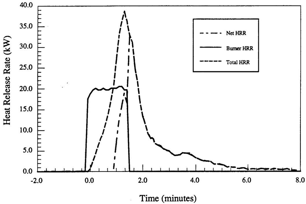
Figure 1.a - Steel - Heat release rate vs. time
