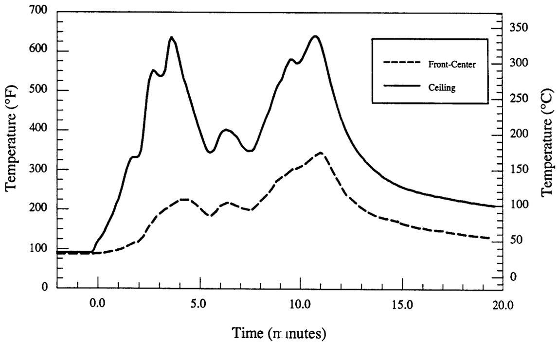
Figure 5.d - Material # 3 - Double chair - Room temperatures vs. time
