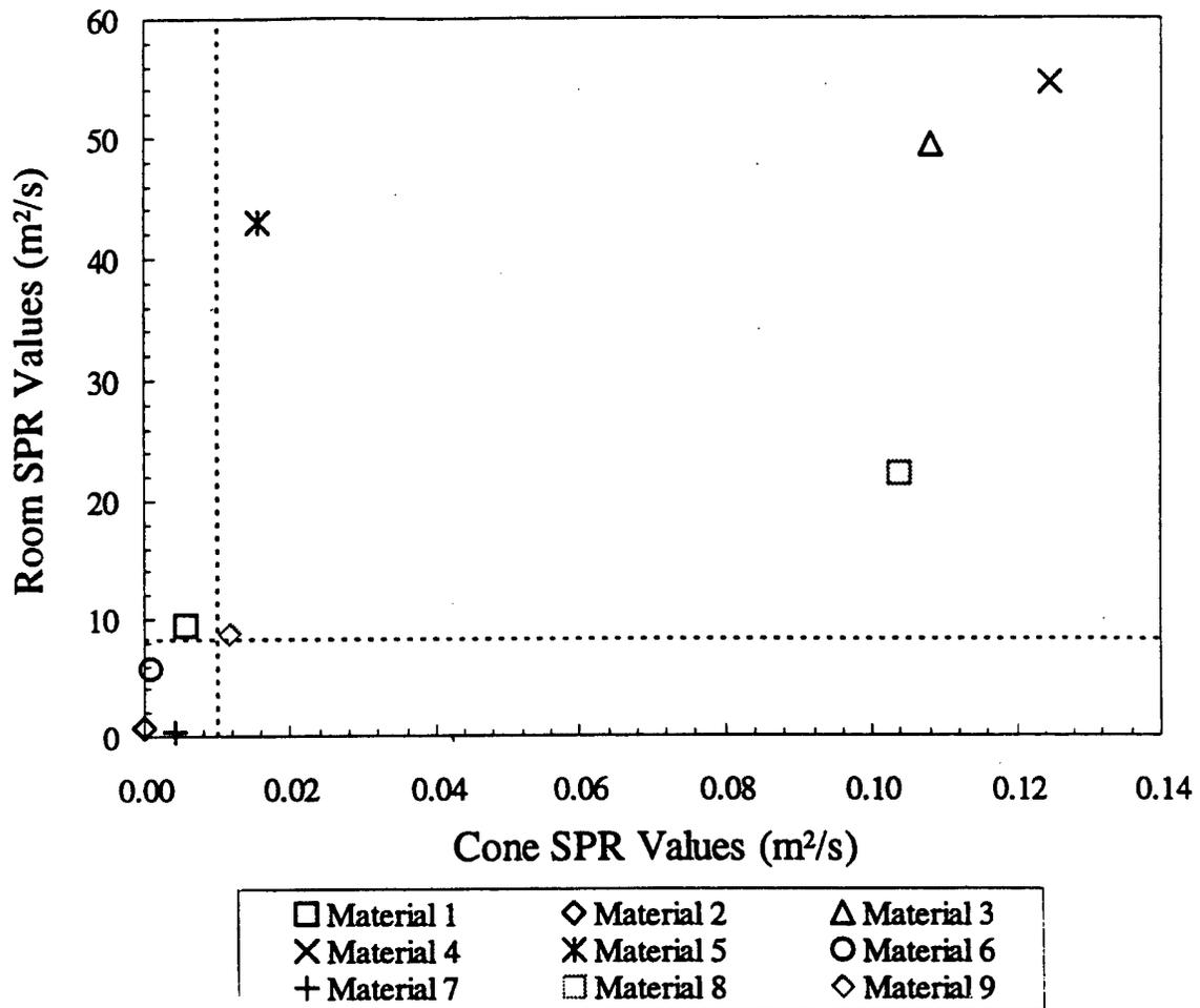
**Figure 8.4 - Correlation of Maximum 60-Second Sliding Average Smoke Production Rates**
