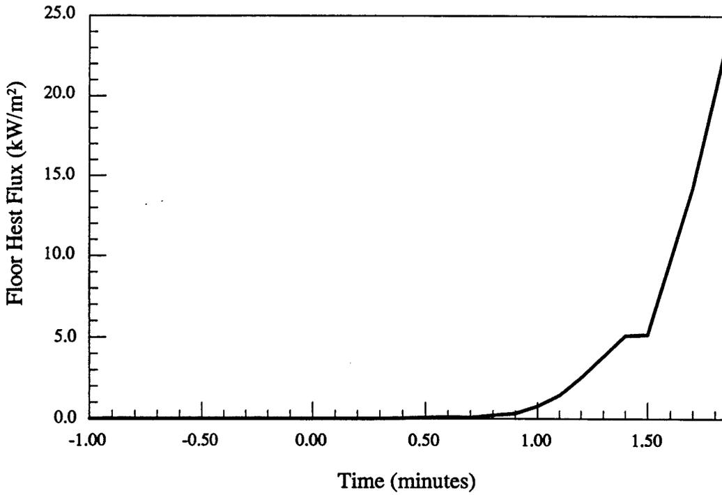
Figure 8.c - Material # 8 - Floor heat flux vs. time
