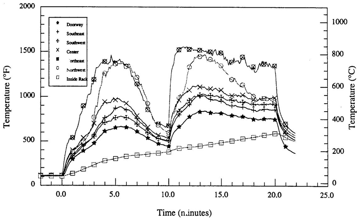
Figure 13.d - Material # 5 - Luggage rack - Room temperatures vs. time
