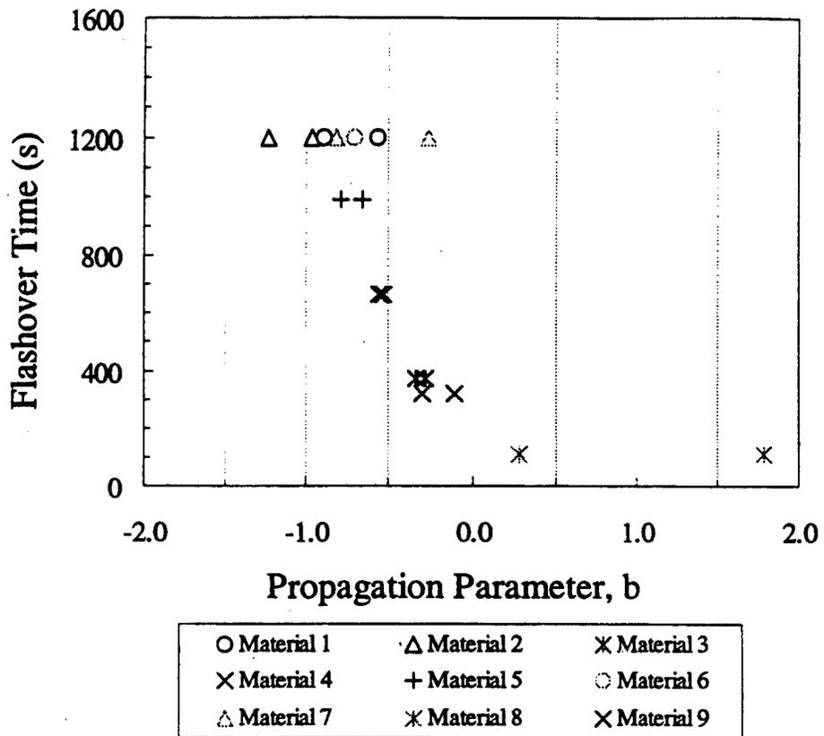
Figure 8.2 -ISO 9705 Flashover Time as a Function of the 75 kW/m<sup>2</sup> Propagation Parameter
