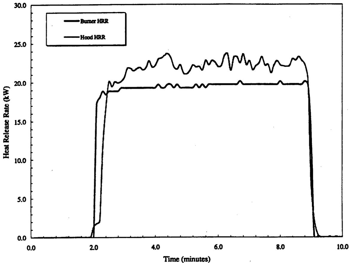
**Figure 4.1 - Comparison of Heat Release Rate for Burner and Exhaust Hood Calculated from Calibration Data Obtained Prior to Furniture Test Series**
