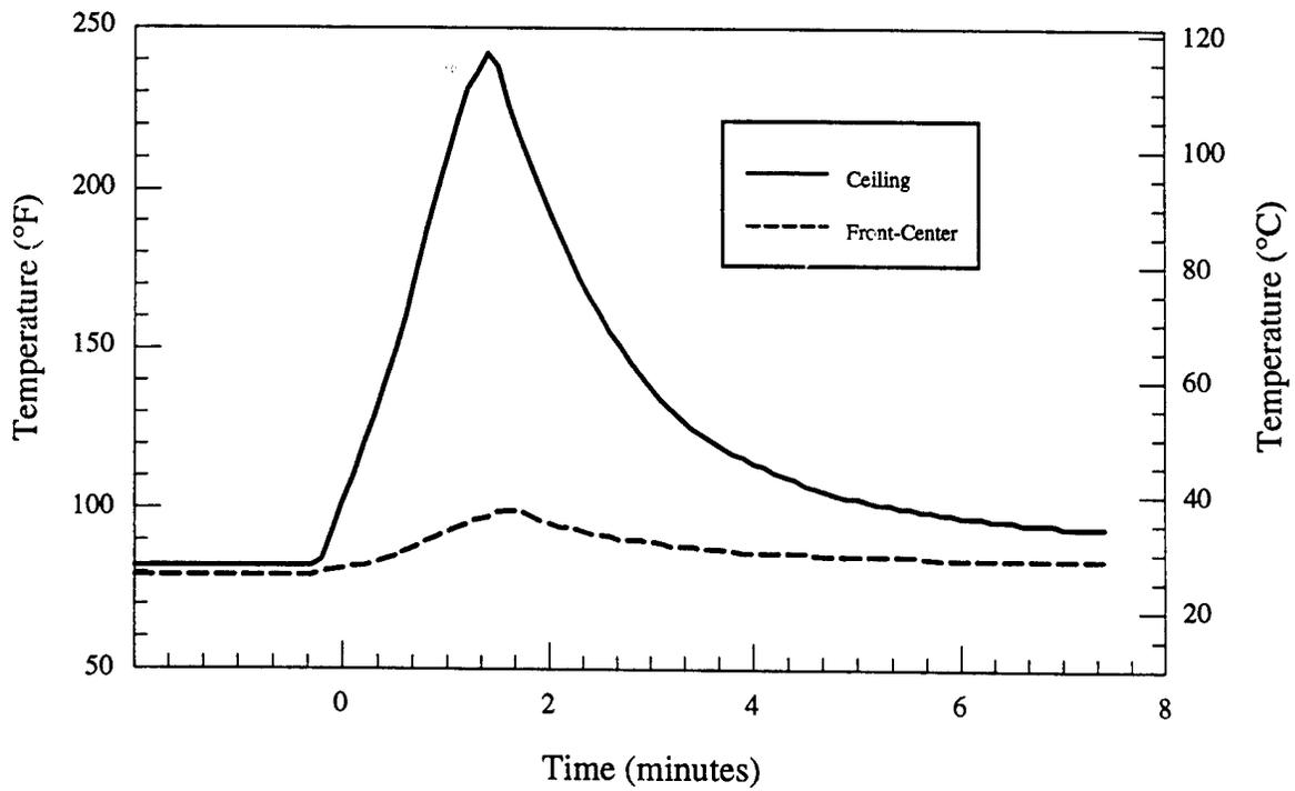
Figure 7.d - Material # 5 - Single chair - Room temperatures vs. time
