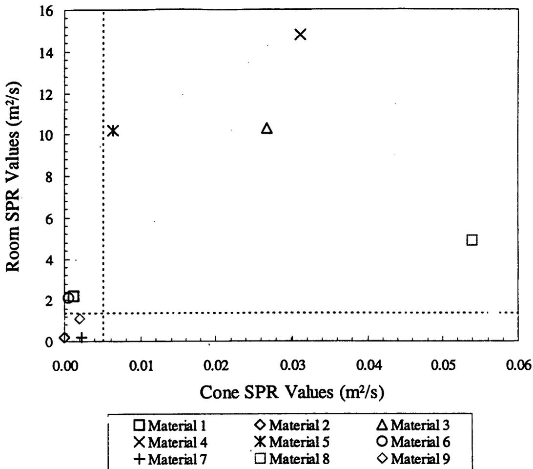
Figure 8-3 – Correlation of Test-Average Smoke Production Rates
