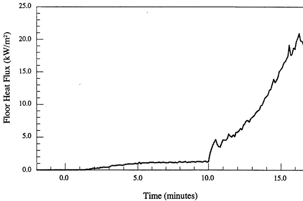
Figure 5.c - Material # 5 - Floor heat flux vs. time
