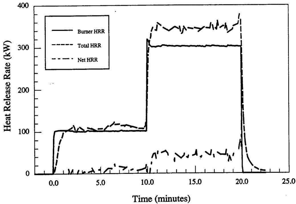
Figure 7.a - Material # 7 - Heat release rate vs. time
