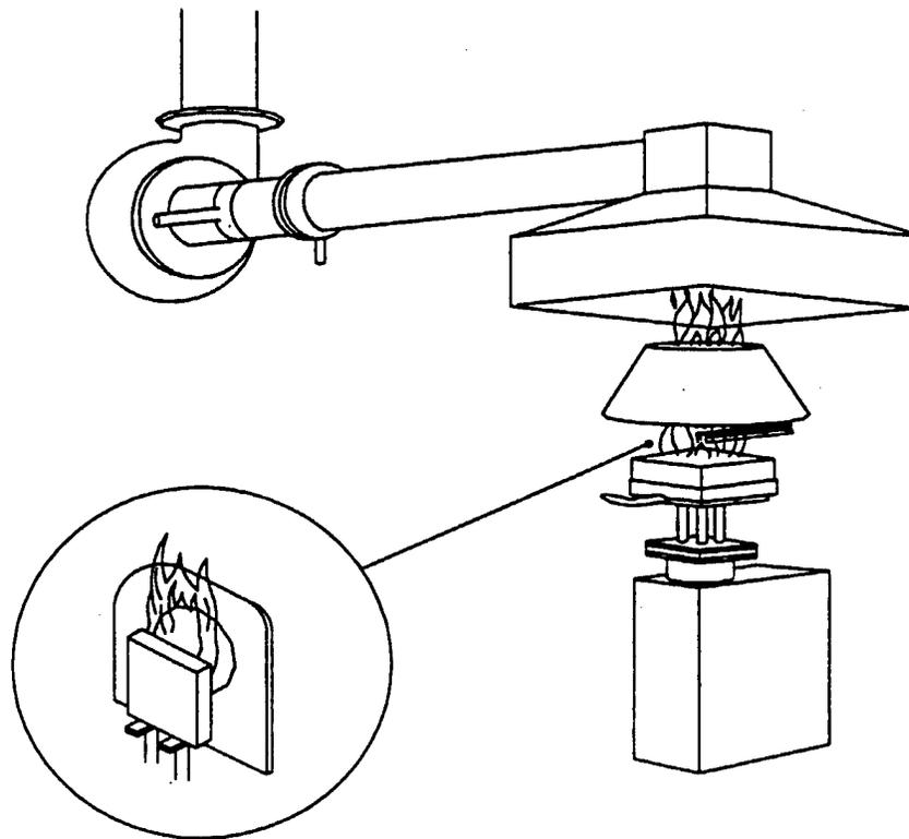
**Figure 5.1 — Schematic of the ISO 5660 Cone Calorimeter**
