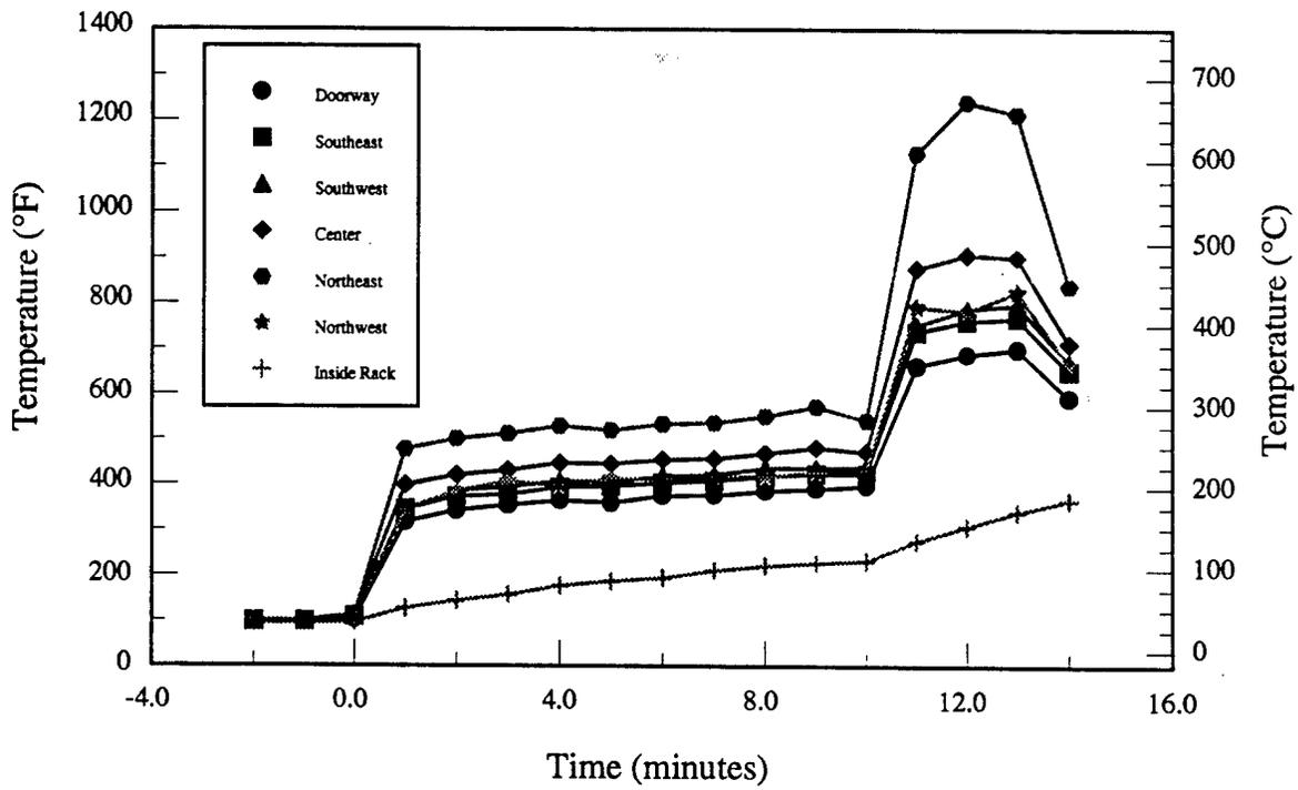
Figure 10.d - Material # 1 - Luggage rack - Room temperatures vs. time
