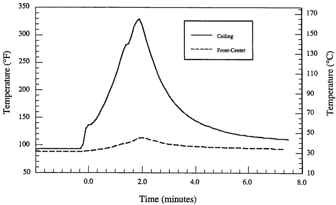
Figure 4.d - Material # 1 - Double chair - Room temperatures vs. time
