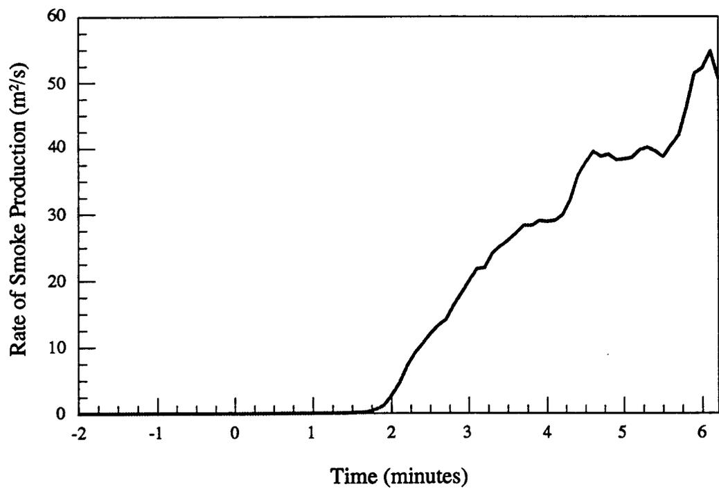
Figure 3.b - Material # 3 - Smoke production rate vs. time
