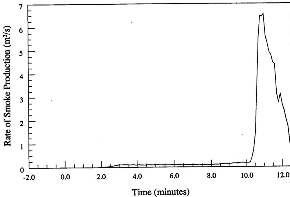
Figure 9.b - Material # 9 - Smoke production vs. time
