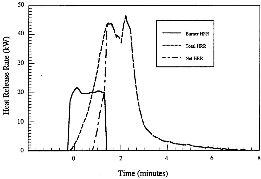
Figure 3.a - Material # 1 - Single chair - Heat release rate vs. time
