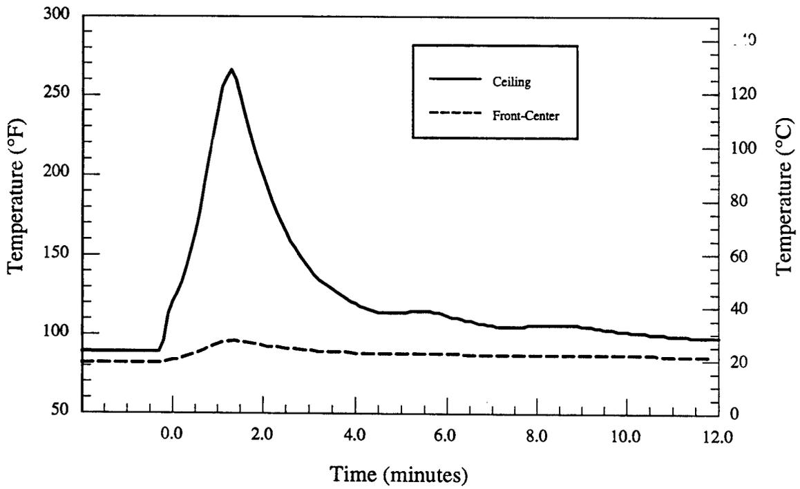
Figure 8.d - Material # 5 - Double chair - Room temperatures vs. time
