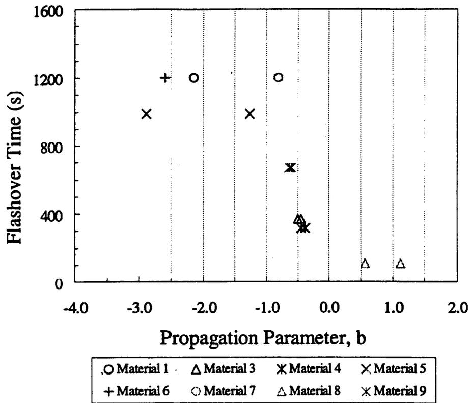
Figure 8.1 – ISO 9705 Flashover Time as a Function of the 50 kW/m<sup>2</sup> Propagation Parameter
