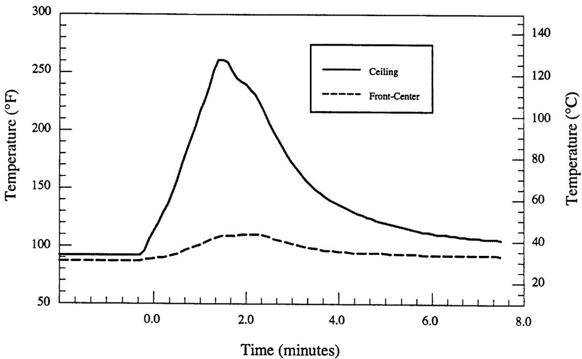
Figure 3.d - Material # 1 - Single chair - Room temperatures vs. time
