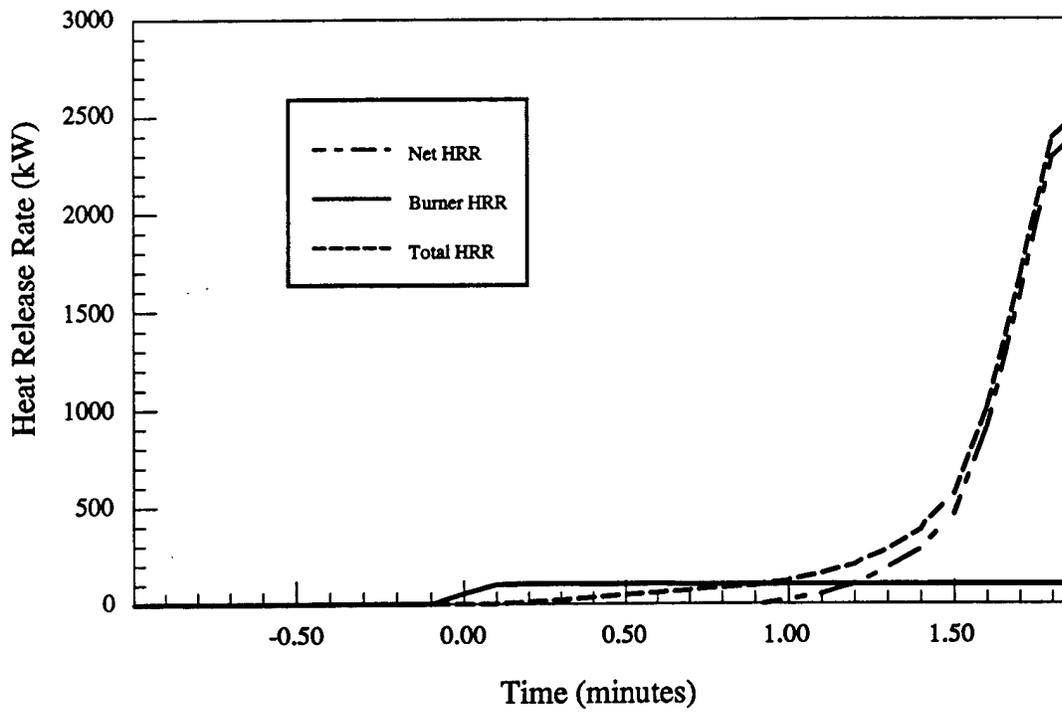
Figure 8.a - Material # 8 - Heat release rate vs. time
