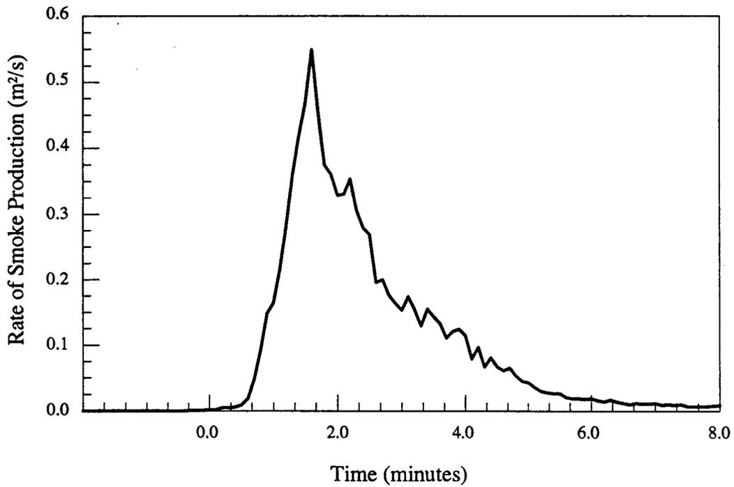
Figure 1.b - Steel - Smoke production rate vs. time
