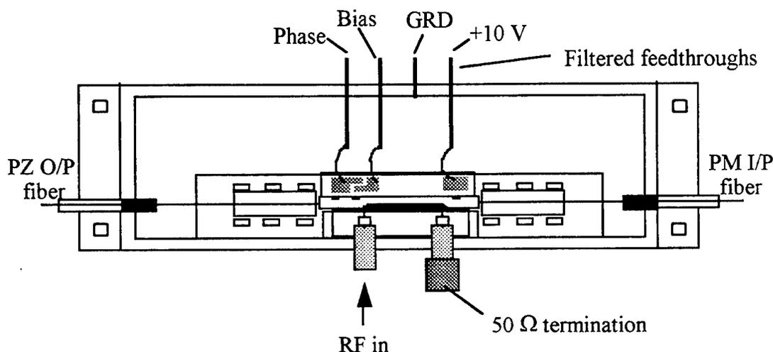
Fig 3.10: Packaged SSB Modulator
