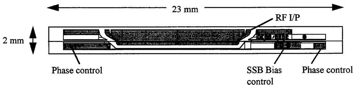
Fig 3.8: SSB Modulator Chip design
