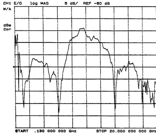
Fig. 3.19: Measured frequency performance of delivered SSB Module
