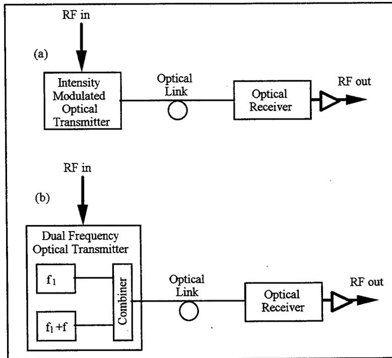
Figure 2.2: Two basic types of optical microwave link
