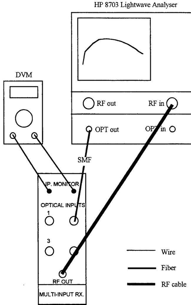
Figure 3.22: Experimental set-up used to assess MIR module
