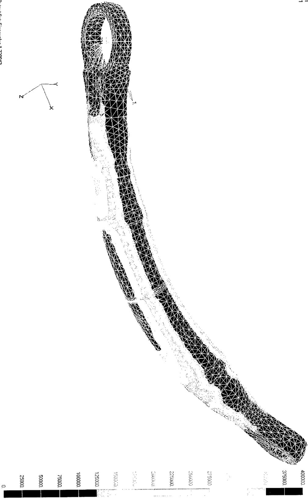
Figure V-1. Nominal Drag Strut MSC/NASTRAN Elastic Buckling Analysis Results.
