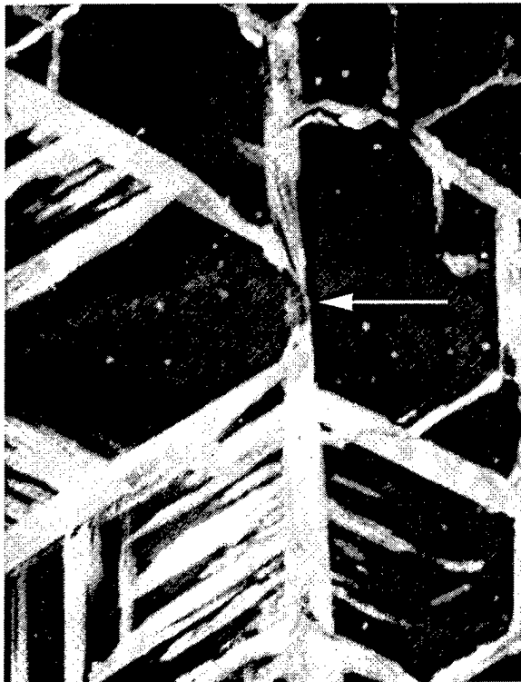
Fig. 2. Fractured disk and close-ups of the fracture initiation site and fracture surface.
