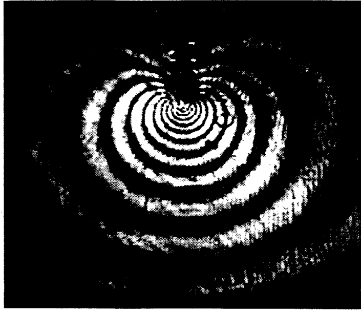
Fig. 3.1.5: Three-point bend of PMMA plate with pre-cut crack.
