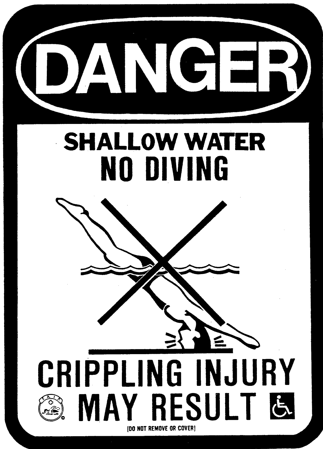
Figure 6-2. A typical sign which should be posted in areas having a water depth less than 5 ft (1.5 m). The word DANGER should have a bright red contrasting background. This sign may be reduced to a 4 in. by 6 in. sign and mounted on the coping of the swimming pool.
