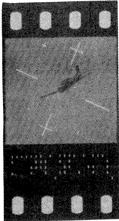
Figure 2. Kinotheodolite photo with coded data
