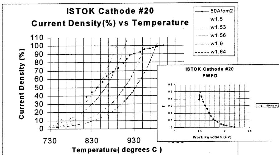
**Figure 5 Emission data for ISTOK oxide cathode.**
