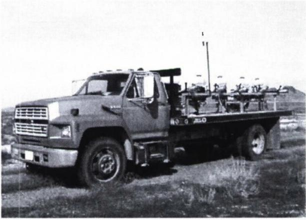
Figure 1-6. Layout of the JFT-4 field trials and photograph of bacteria dissemination truck showing four agricultural sprayers mounted on right-hand side of truck bed.
