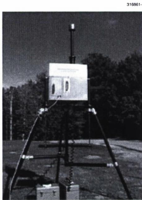
*Figure 1-1. Bioaerosol fluorescence sensor at Lincoln Laboratory. The sensor is completely contained in the silver box mounted on the black tripod. The tube extending 2 ft above the sensor samples air at the same height as the truth sensors (see Figure 1-7). The sensor is shown powered by two battery boxes sitting on the ground.*
