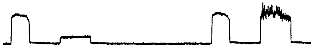
(c) Input pulse sequence and echo signal. Full horizontal scale = 102.4 \mu\text{s} . The duration of the data pulse is 10 \mu\text{s} (400 bits). The input pulses are attenuated by \sim 10^{-4} .
