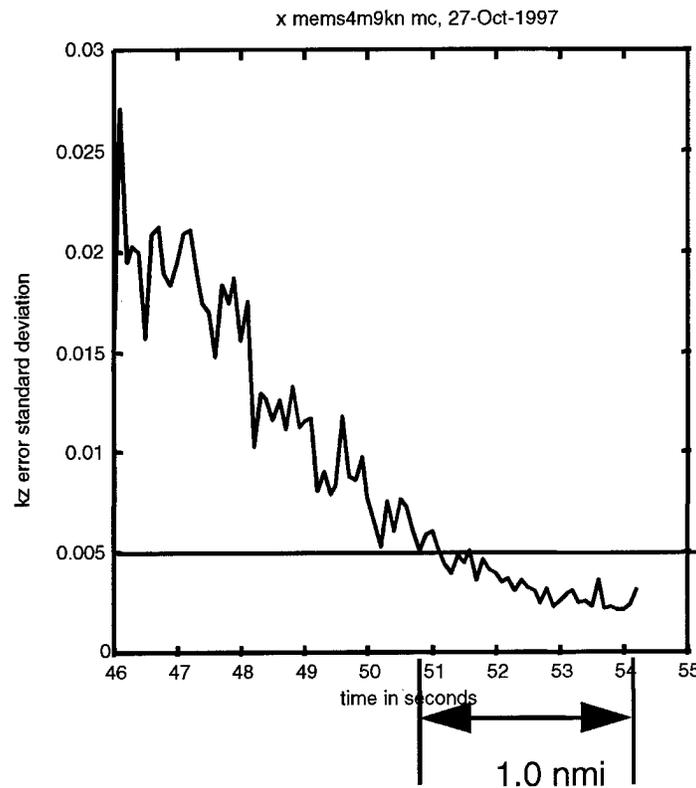
**Figure 10. X-Band Elevation Angle Error vs. Mission Time**
