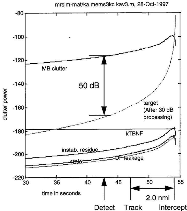
**Figure 11. Ka-Band Seeker Performance vs. Mission Time**
