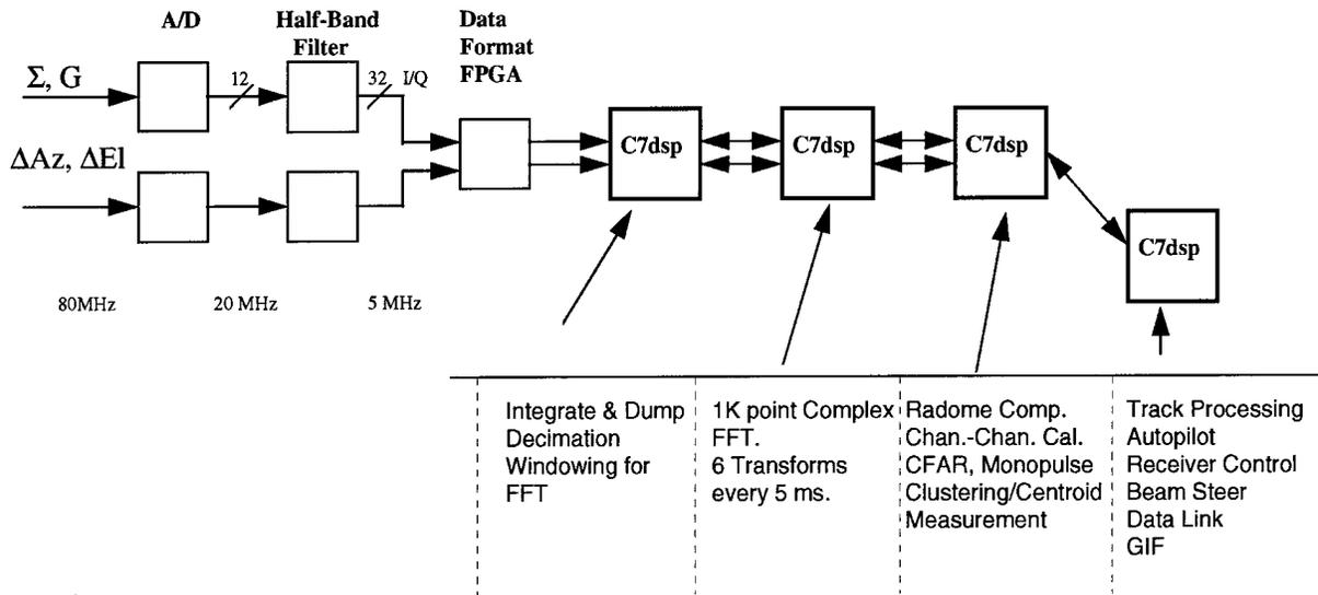
**Figure 17. X-Band Digital Processor Functional Block Diagram**
