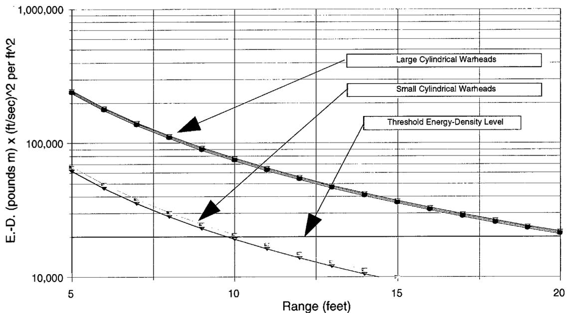
Figure 23. Energy Density vs Range for Cylindrical Warheads
