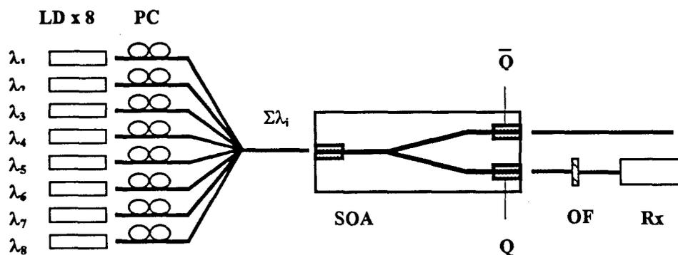
Fig 14 Exnerimental setup PC: nolarization controller OF: ontical filter LD:
