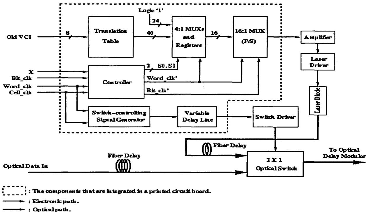
Figure 4 Block Diagram of the VCI-overwrite Unit
