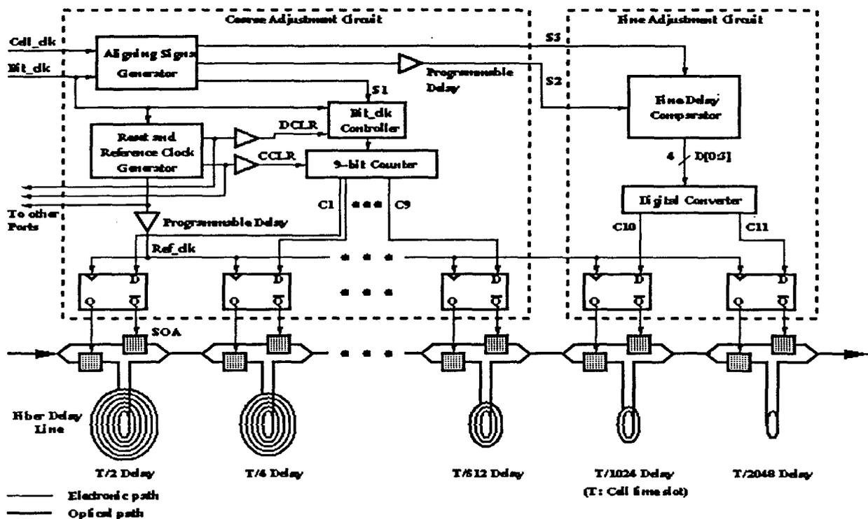
Figure 5 Block Diagram of the Cell Synchronization Unit
