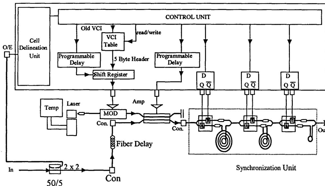
Fig. 2 Architecture of the Photonic Front-End Processor
