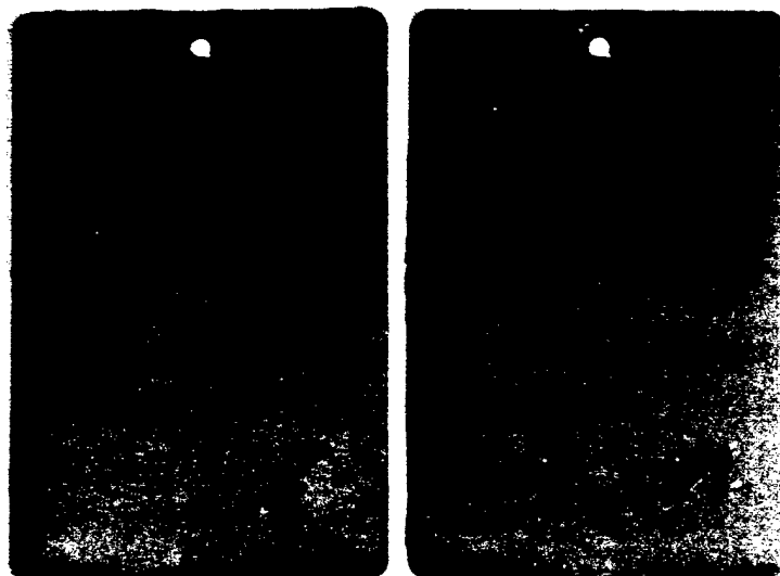
SILICONE ADHESIVE WITH EPOXY SYSTEM 2 Month Marine Atmosphere Exposure
