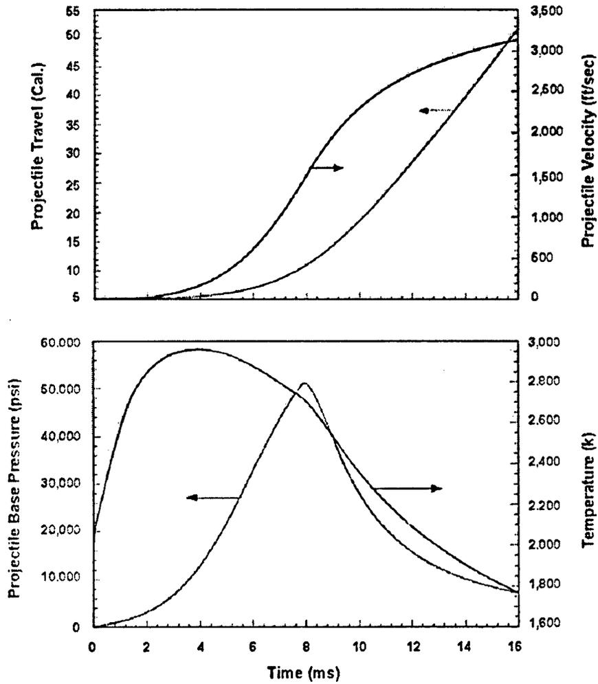
Figure 3. Simulation of inflow boundary conditions for M549A1/XM230/Zone 6.
