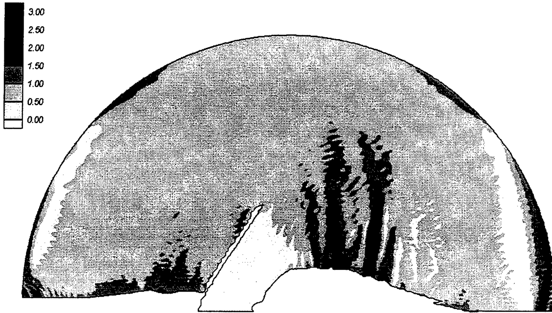
Figure 25. Estimated wave height diagram for normal incident direction, 15-second period wave condition
