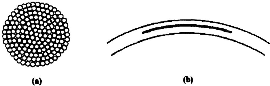
Figure 1: A schematic of an intrastromal femtosecond laser cut. (a) The front view of the intrastromal spiral disk pattern. (b) The side view of the spiral pattern within the cornea. Note that the size of the bubbles is about 120 times smaller than the thickness of the cornea.
