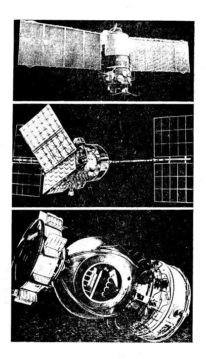
Top: One of the exhibits in the pavilion: the space weather explorer, the satellite "Meteor-2." It ensures collection of meteorological information and its transmission to the earth.
