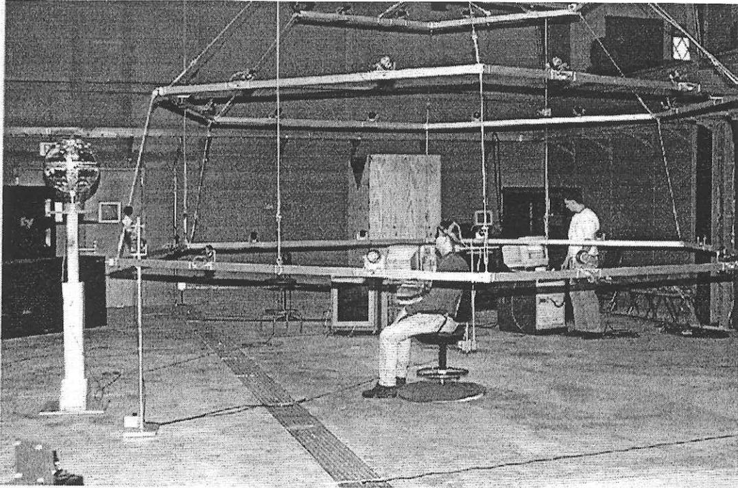
Figure 2. Speaker array, 360° azimuth, for baseline localization accuracy.
